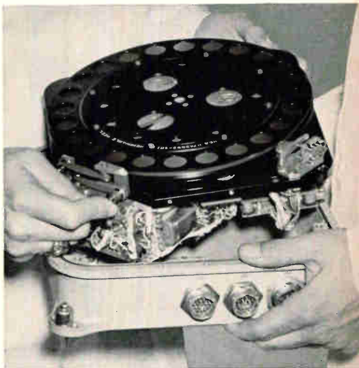
The miniature recorder-reproducer designed for the two-man Gemini spacecraft, weighs 14.5 pounds and uses only 12.5 watts of electric power.
