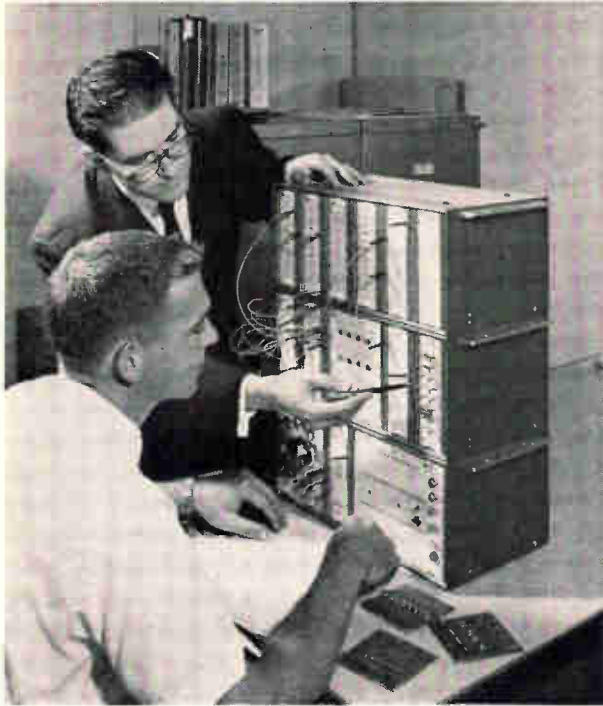
Breadboard and training kit, by Packard Bell, has circuit cards that are plugged into adapters.
