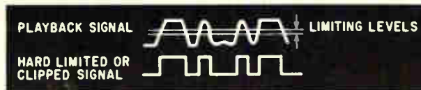
Hard-limiting results in regeneration of the playback signal.
