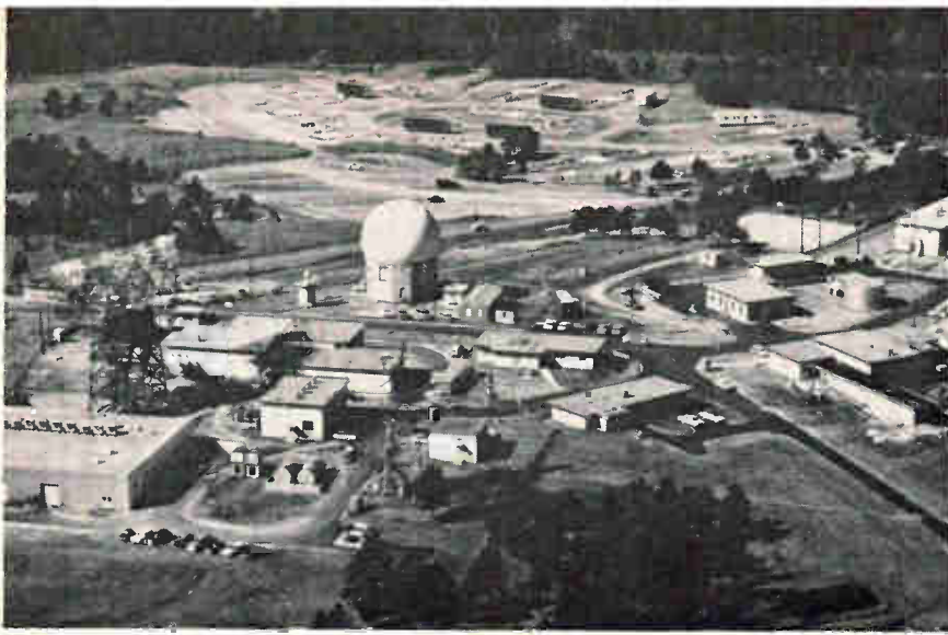
These frequency-diversity type radars, used now in the electronic counter-measures test range, will also be used for the new weapons effectiveness tests. The radar with the round radome is the AN/FPS-26, the large, exposed dish is the AN/FPS-24.
