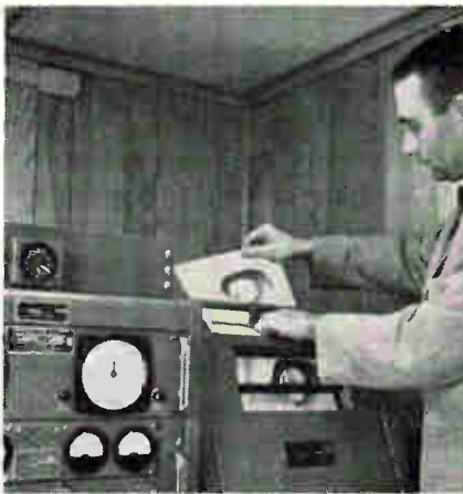
Test readout is taken from a Fairchild-Stratos commercial station by Charles M. Hunter, Spacecraft Manager of NASA's Tiros Operational Satellite program. Hunter and Edward Rich Jr. describe on page 81 how to assemble a low-cost ground station.
