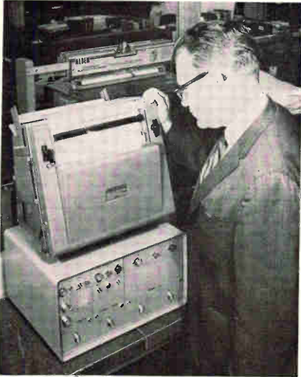
Paper facsimile recorder is Alden dual mode model 9225. Muirhead and Fairchild Camera machines also may be employed.
