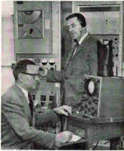
Ottawa station uses a scope for display, instead of a facsimile machine. R.S. Rettie of Canada's National Research Council, adjusts receiver while C.I. Taggart of the Meteorological Branch of the Department of Transport watches the signal on oscilloscope.
