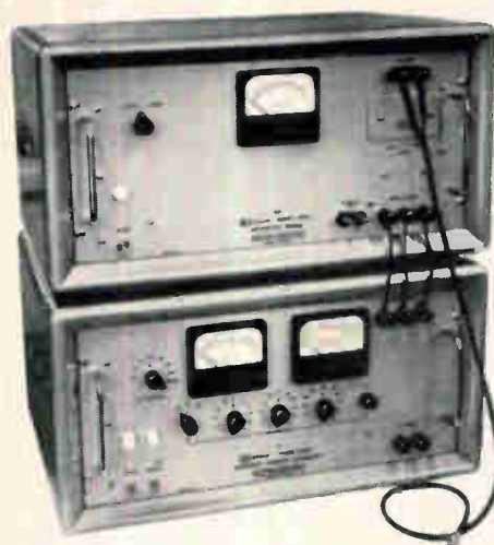
Models 1493-1 1494-1 Bolometer Bridge and Reference Current Generator—provides automatic measurement of microwave power with \pm 0.1\% accuracy. Supplied for standard rack mounting or with individual cases.
