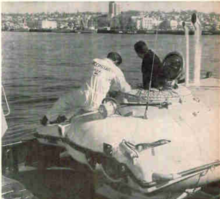
Diving Saucer, being prepared for a test at San Diego, Calif., has a 1,000-foot capability.
