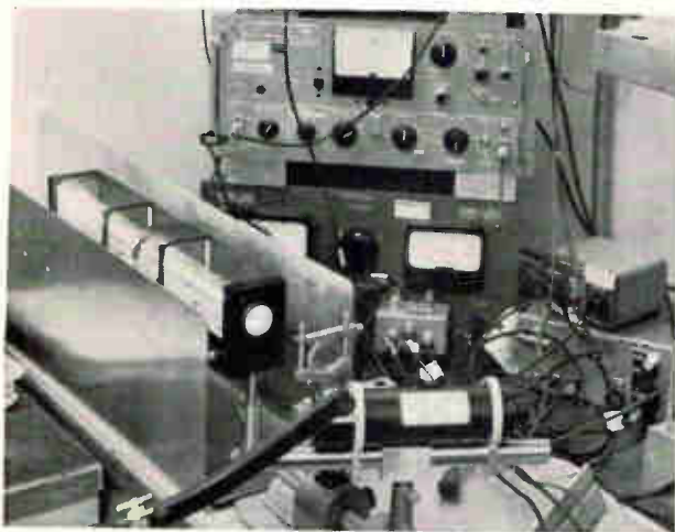
Test setup of an 11-to-20-gigacycle traveling-wave phototube and helium-neon gas laser.
