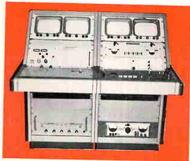
Remote station has multiple displays and an operator's joystick.
