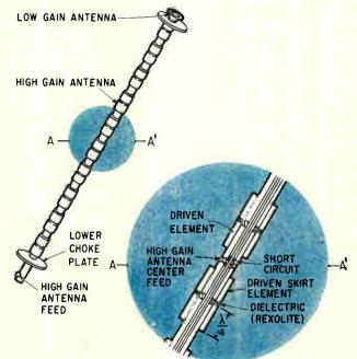
High-gain antenna is 10-element series fed collinear array of stacked dipoles; low gain antenna is a discone type fed by a coaxial line through the center of the high gain antenna
