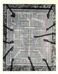
Two-stage differential amplifier was designed with computer techniques. Note the arrangement of circuit elements about a vertical line of symmetry
