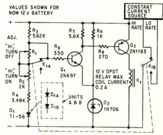
After system primary power is restored, this controller recharges batteries in 20 hours, provides trickle charge
