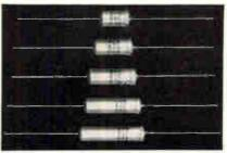
You can get a lot of capacitance ... and a lot of quality ... in this compact-size line of aluminum case electrolytics. Designed especially for transistorized equipment, the TCW series has a combination of excellent stability and economical price which makes them a leading choice in industrial and entertainment equipment. Long service life is assured by all welded construction, with positive end seal. Leakage current and ESR are uniformly low and stable.
