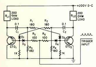
GTO adaptation of the SCR capacitor-commutated flip-flop transfers load current each time a positive trigger pulse is applied
