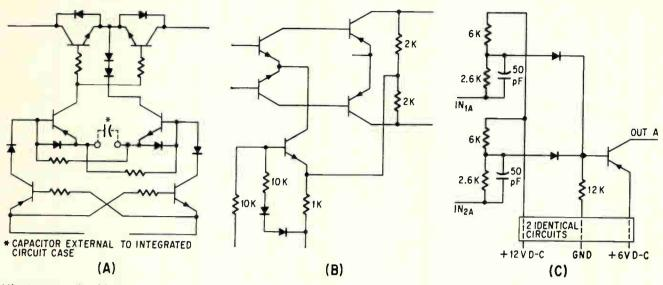
Minuteman units. These are the demodulator-chopper (A), a general-purpose amplifier (b) and matrix switch (c) that Autonetics designed for the improved Minuteman missile
