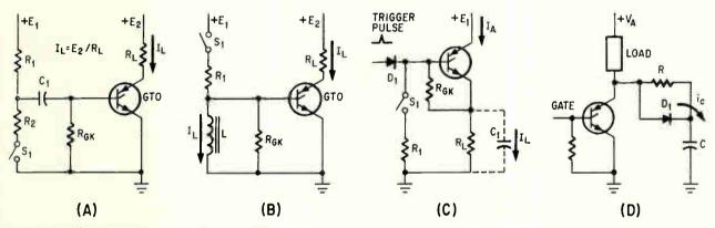
Four turn-off methods for controlling the GTO. Device may be turned on and off by charging and discharging a capacitor in series with gate lead (A). Turn-off is achieved by interrupting d-c current in inductor between gate and cathode (B). Load impedance is connected between the GTO's cathode terminal and ground (C). Use of capacitor C allows higher anode current switching by diverting part of the anode current (D)
