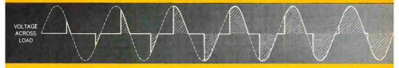
The newest member of Transitron's BiSwitch family, the 11/16'' stud-mounted TBS40AS. handles up to 20 amperes at 125 volts. It gives direct full-wave AC phase control of 2.5 KW. And no AC to DC converters or variacs are needed. It permits high power control circuitry that is simpler, more reliable and more economical than ever before possible.
