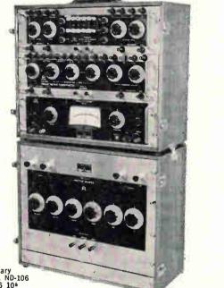
Julie portable DC primary standards laboratory: PRB-205 Primary Resistance Bridge, PVP-1000 Primary Voltage Potentiometer, ND-106 Null Detector, VDR-106 10<sup>4</sup> Voltage Divider.
