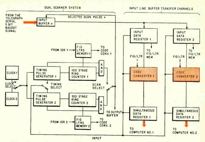
Input block diagram (left) shows special features of the electronic telegraph system front-end design. Incompatibility between conventional teleprinter signaling code and
