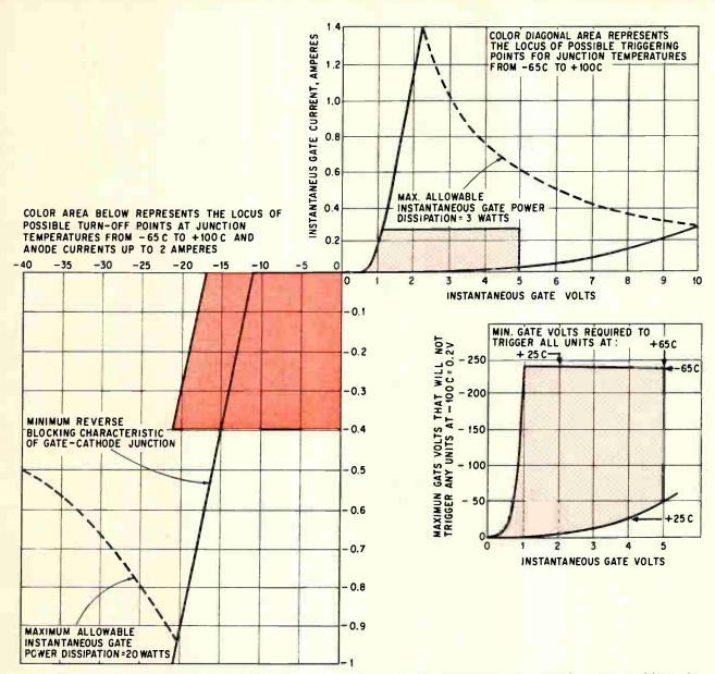
Gate triggering characteristics are needed to design circuits using GTOs. The first quadrant defines the positive gate triggering voltage-current relationship while the third quadrant displays the equivalent negative turn-off data
