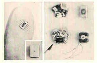
Monolithic amplifier, old circuit and earphone (top); microphone, new circuit and telephone coil (bottom)
