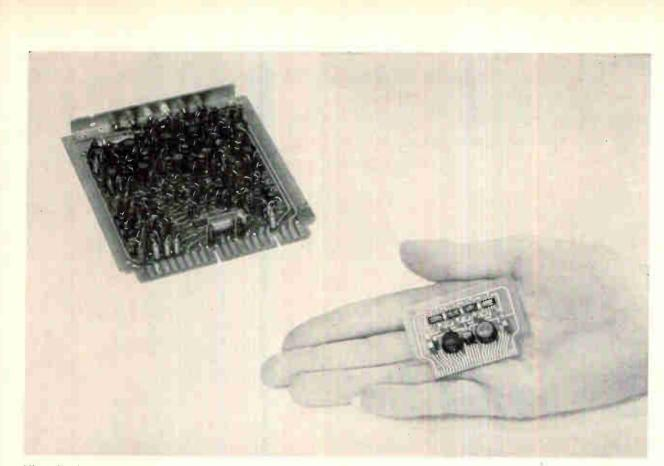
Microcircuit version of frequency tracker audio circuit replaces printed board version that uses discrete components
