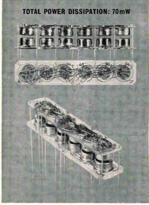
Three views (actual size) show high density assembly of circuits in TO-5 type packages.
