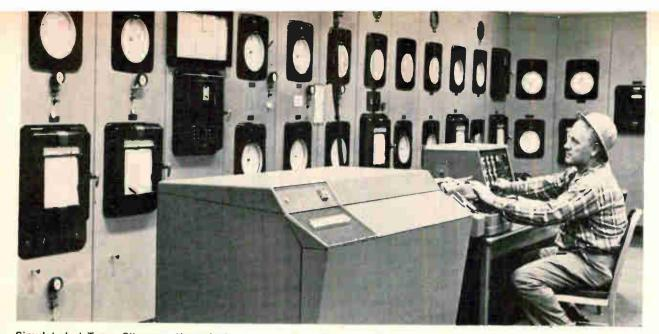
Simulated at Texas City were those instruments at the left next to the air gages. Tests using an RW-300 computer proved DDC'd loops responded at least as well as conventional loops but in most cases both smoother and faster
