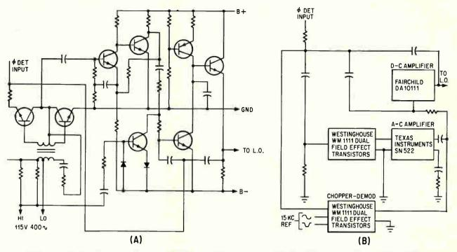
Integrator's conventional circuit (A) uses chopper transistors in pairs while the MIC version (B) uses field-effect transistors to handle chopping and demodulation
