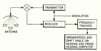
Self-contained doppler navigation system consists of four principal electronic blocks—transmitter, receiver, frequency tracker and computer
