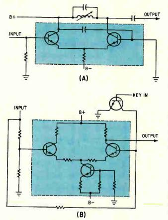
Receiver requires external adaptive circuits (A) for the 30-Mc amplifier stage. The suppressed carrier double-balanced modulator (B) has achieved a carrier rejection of 40 db. MICs are in color
