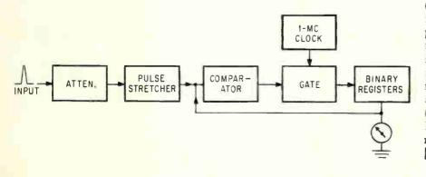
ured with this instrument. Model 5201A is considerably more simple to use than an oscilloscope for these applications as there are no sync, gain, triggering level, sweep speed nor other controls to adjust. It may be used unattended in applications where transients occur at random.
