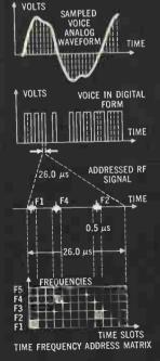
\* RADEM (Random Access Delta Modulation) principle diagramed above is the result of 5 years of independent
