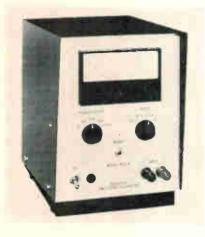
for system checkout, circuit investigation and general lab use, and may also be used for unattended monitoring of power supplies, power lines and life-test systems.
