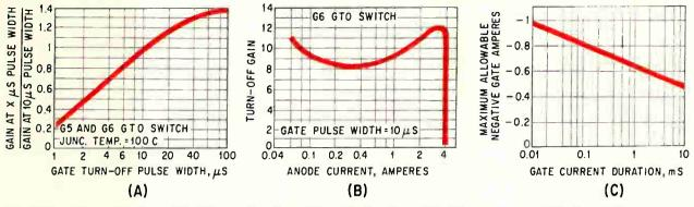
Turn-off gain for type G5 and G6 GTO as a function of the turn-off pulse width (A) and load current (B). Avalanche gate current is plotted as a function of gate pulse width in (C)
