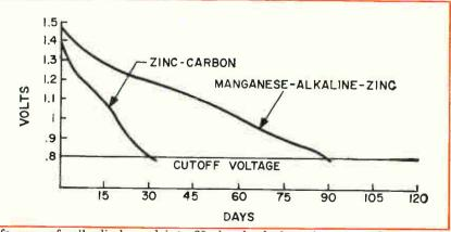
Life span of cells discharged into 60-ohm loads for 8 hours per day at 70°F.
