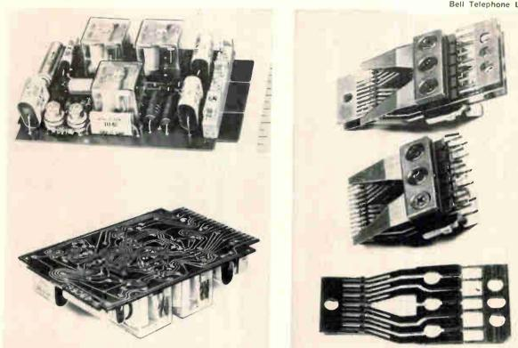
Plug-in printed wiring board with MB type relays
