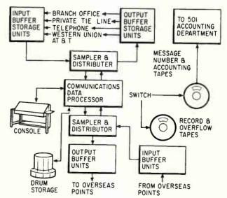
Electronic telegraph system controlled by computer is aided by input-output buffers and storage facilities
