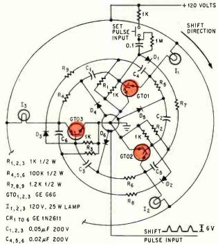
Ring counter may function as decade counter with direct lamp readout
