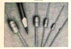
Developed by the Sprague Electric Company to help designers of digital computing equipment and other industrial electronic devices reduce their costs, Type 154D solid-electrolyte Tantalex Capacitors have performance characteristics which are comparable to those of higher-priced metal-clad capacitors from other sources.
