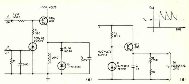
GTO can be used as a high speed hammer driver for a computer readout mechanism (A) and as a free-running high voltage sawtooth generator (B)
