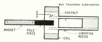
How the tuned relay works
