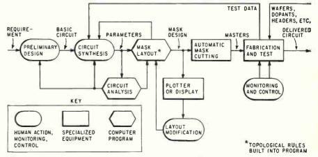
Hexagons show where computer techniques fit into Norden's design and manufacture of microcircuits
