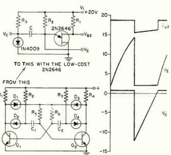
2N2646 FIRING CIRCUIT FOR LOW AND MEDIUM CURRENT SCR'S LOW-COST MULTIVIBRATOR WITH OUTPUT WAVEFORMS
