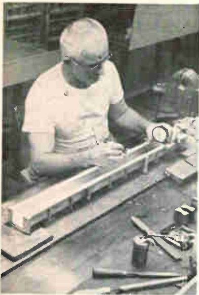
HAND LAPPING was used to obtain critical surface tolerances with old design
