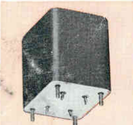
Low frequency band pass filter. Designed for 2.5 cps center frequency. At 2 to 3 cps within 3 db. At 1.5 cps and lower, and 4 cps and higher, greater than 30 db. Source and Load 10K ohms. Size: 4 x 4-11/16 x 6". MA MIL case, MIL-F-18327B.
