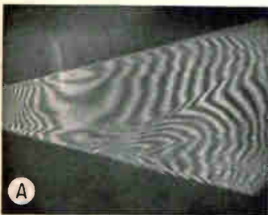
CONVENTIONAL interferogram, (A), was taken with filtered BH-6 mercury arc, air-to-air injection at Mach 2.3 station, 250 psi chamber pressure, 150 psi injection pressure. Laser interferogram (B) shows improved resolution, was taken with argon-to-air injection at Mach 2.3/station (point where flow reaches 2.3 Mach speed) 105 psi chamber pressure, 35 psi injection pressure
