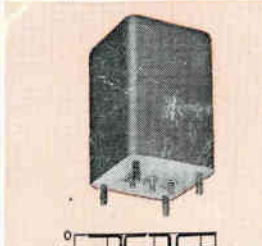
High frequency low pass filter. Zero to 700 KC within 1 db. 1.95 mc to 10 mc 40 db minimum. Source and Load 1000 ohms. Molded flat construction for printed circuit applications. Size: 1 x 2 x 1/2"; Wt: 1 oz. MIL-F-18327B.
