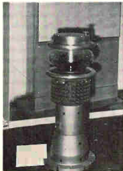
HEDGEHOG EFFECT at middle of tube is the magnet assembly and cooling fins of CSF's Artatron
