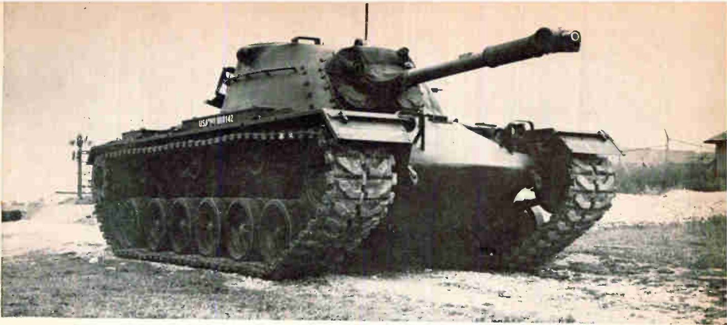
INFRARED photoelectric telescope is mounted in the M-48's gun. Radio antenna and infrared beacon assembly are mounted atop the turret
