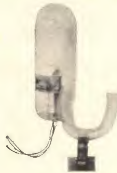
1912—General Electric's Dr. Irving Langmuir developed this early high-vacuum tube useful in establishing laws of electron flow.
