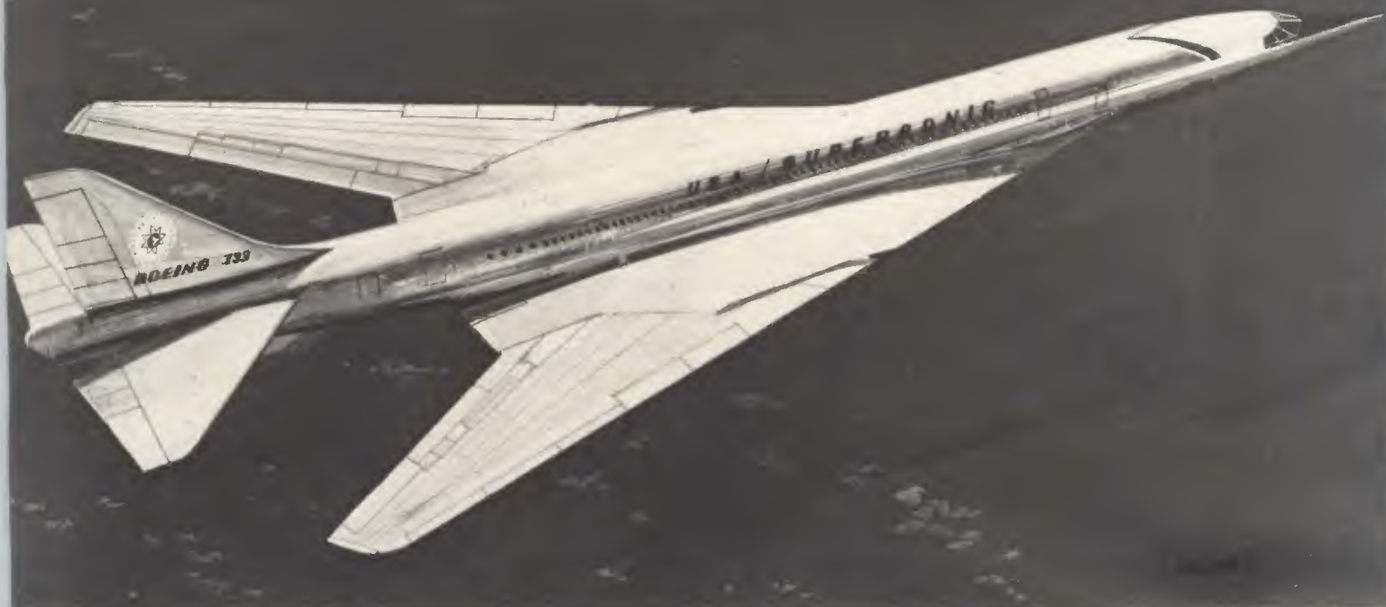
Lockheed and Boeing entries in the supersonic race. The Boeing "variable-sweep" supersonic transport is shown above.
