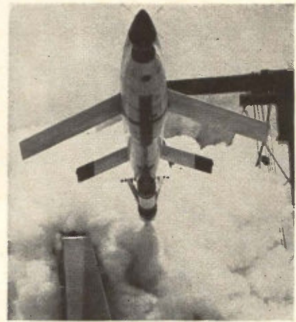
Helicopter pilots in search of drones, like the Firebee Q2C, downed in the water would like some help. They suggest a radio beacon in the drone.
