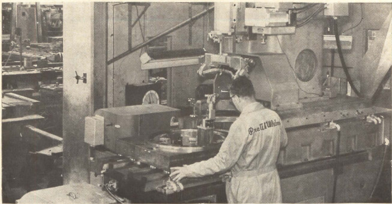
Ballistic missile nose cones are among thousands of items being measured daily with numerically controlled inspection machines. Here the operator checks positioning of the inspection probes on a Pratt & Whitney six-coordinate measuring machine.
