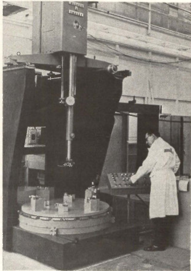
Turbine blades and other complex rocket engine parts are inspected on this Warner & Swasey three-coordinate machine at the Douglas Aircraft Co. in California. The base and parallel vertical black sides are of granite. This is one of the largest inspection machines ever built.
