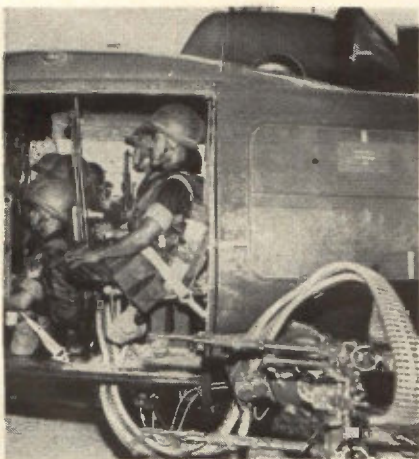
Army helicopter loaded with Vietnamese paratroopers. Twin machine-gun mount in foreground is part of M6 armament system.
