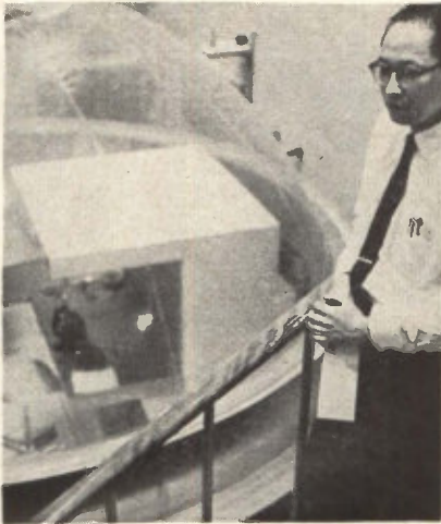
Plastic bubble behind Ko is a clean room. Protective films filter out ultraviolet light.
