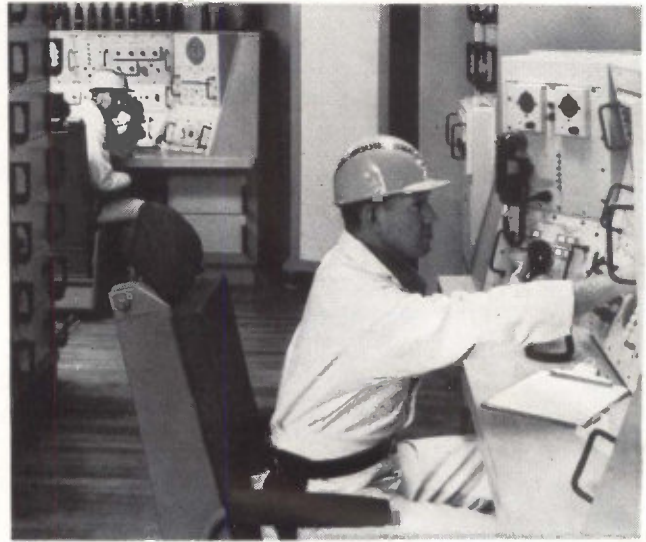
FULL-SCALE mockup of instrument panel for underground launch control center
