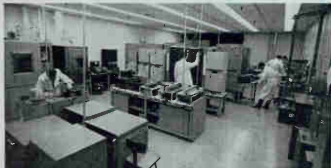
The TRIMPOT Division Environmental Laboratory is capable of performing tests to MIL-R-27208, MIL-R-22097 and MIL-R-12934.
