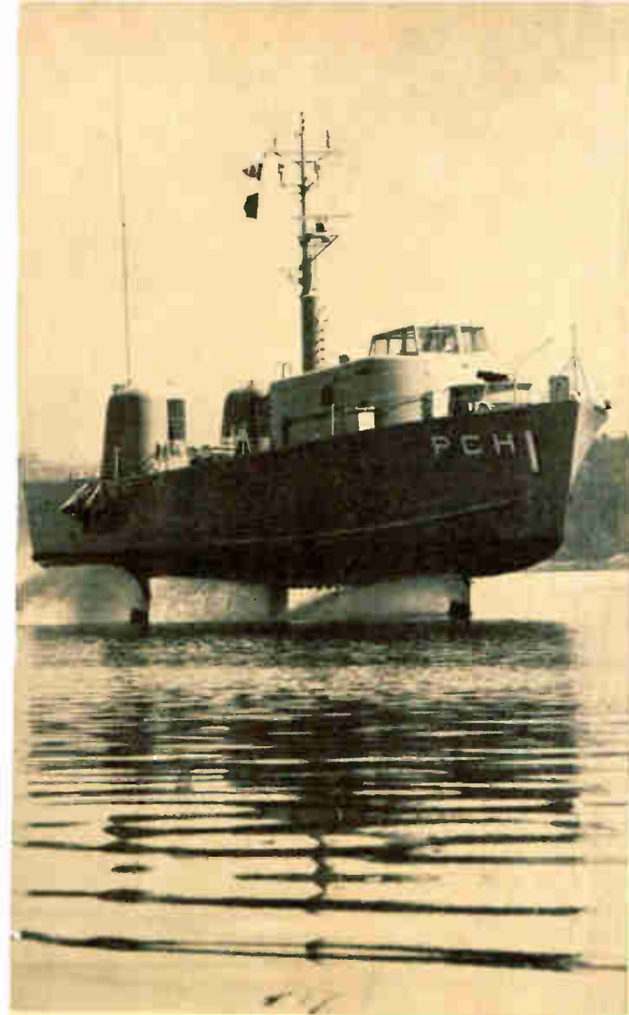
ANTISUBMARINE DUTIES may evolve for a class of hydrofoil boats designed to "fly" above the surface at speeds over 100 knots. Boeing developed this craft, which uses electronic stabilization of submerged foils
