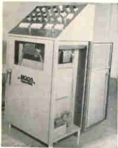
CONTROL CONSOLE has key board for operator to set in drilling coordinates. Tapes are reused for each work piece
