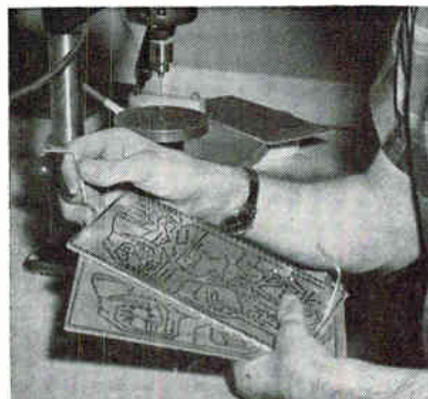
DRILLING TEMPLATE made by same master on aluminum or steel provides accurate positioning of required holes for components
