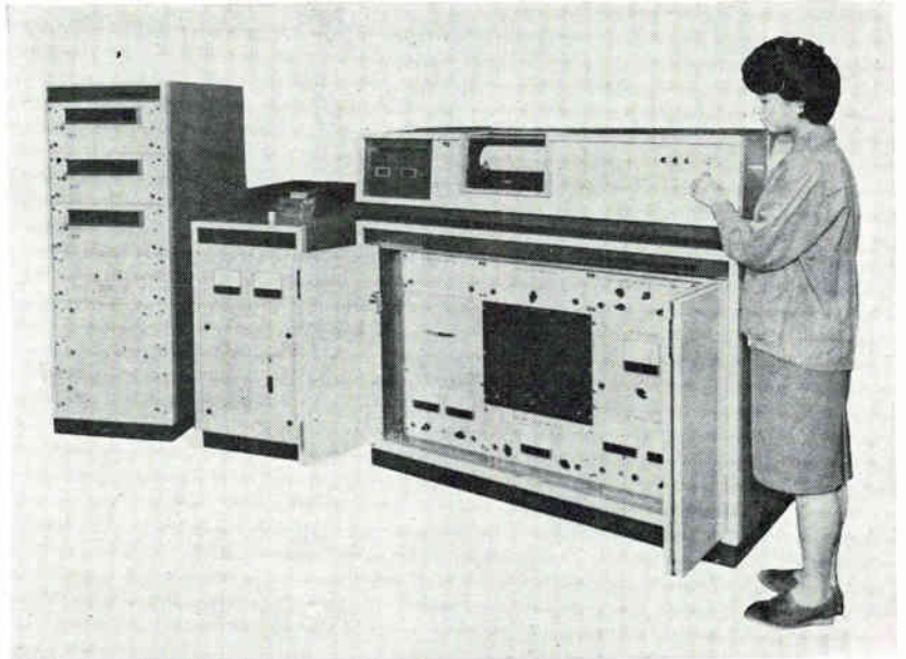
COLOR COMPUTER comprises four major units: electronic tristimulus integrator with digital tube display, extreme left; voltage stabilizer and output printer, center, optical portion of recording spectrophotometer, top right, and electronic portion of recording spectrophotometer, bottom right
