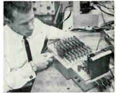
NBS ENGINEER Owen Laug inserts probe of tester into self-test receptacle of fault-location test set
