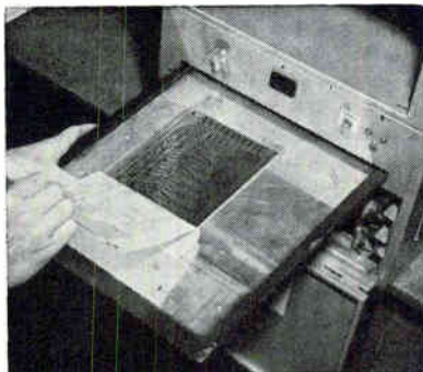
DRY IMAGE of circuit is transferred from paper to copper in processor to produce chemical resist pattern
