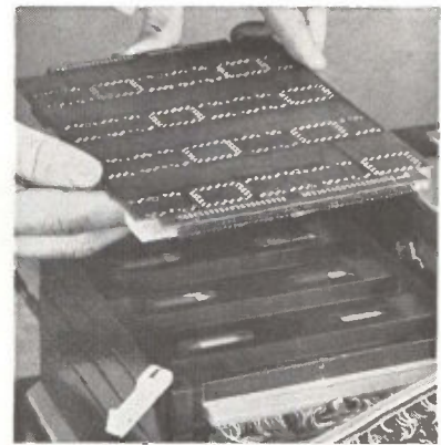
COMPUTER for new guidance system uses welded-wire circuit modules assembled on printed-circuit laminates and stacked on heat-conducting trays next to drum memory
