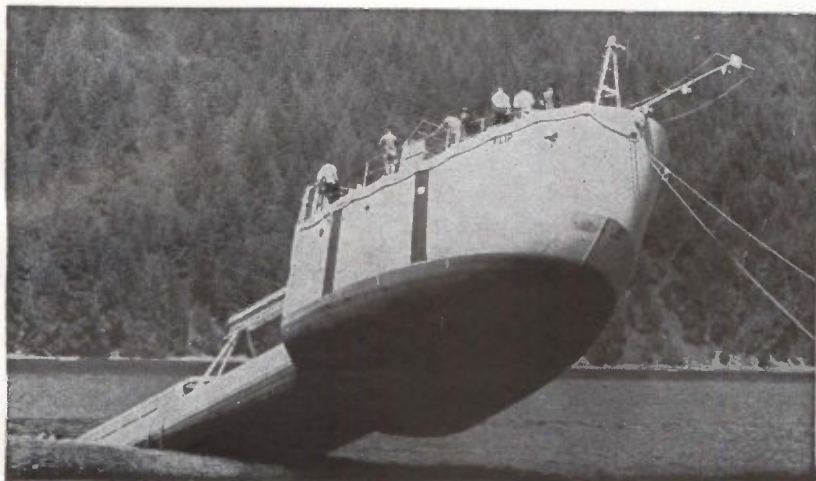
FLIPPING into vertical position is Flip (Floating Instrument Platform), an important tool for making accurate measurements of sound transmission in the ocean and for other tests important for ASW work. Total Navy spending for oceanography in 1964 will be $106.9 million. Other government agencies will spend an additional $82.5 million
