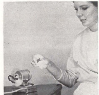
LIGHT from match activates photo-cells to operate motor
