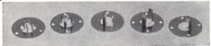
ANODE VANES of magnetron tubes produced by electric discharge machine have tolerances of \pm 0.0001 inch
