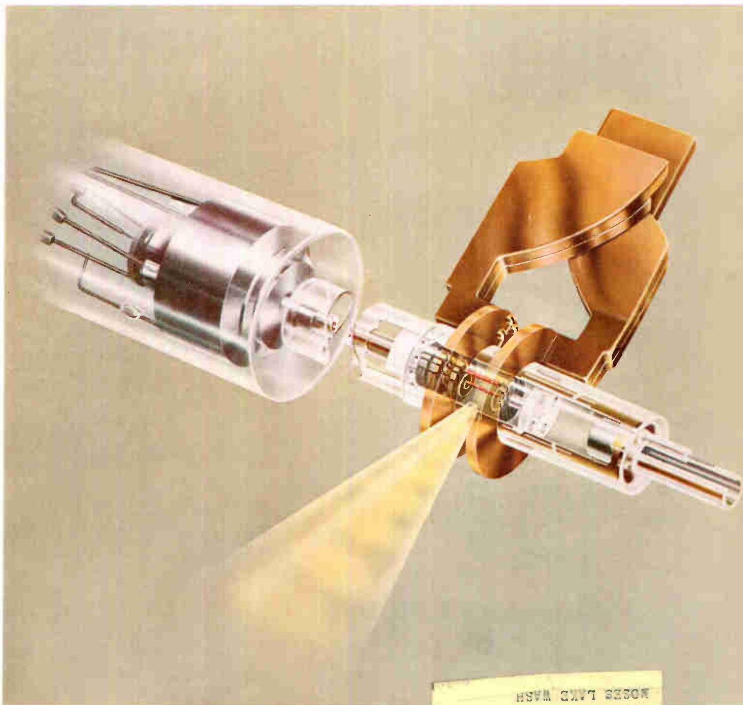
TORNADOTRON, a generator for one-millimeter waves, p 21
