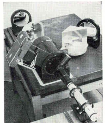
CONTINUOUS WAVE gas laser in ring mount, foreground, emits beam passing through interferometer and then reflected through prism under test, right. Optical fringes are observed in eyepiece on interferometer
