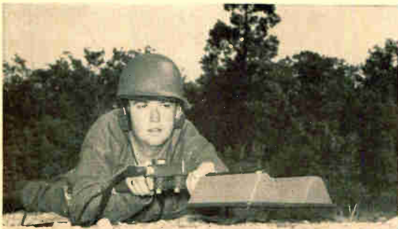
FIRST PHOTOGRAPH of microwave mine detector (p 8, Aug. 9) released by Army last week. Device detects metal, plastic and wooden mines
