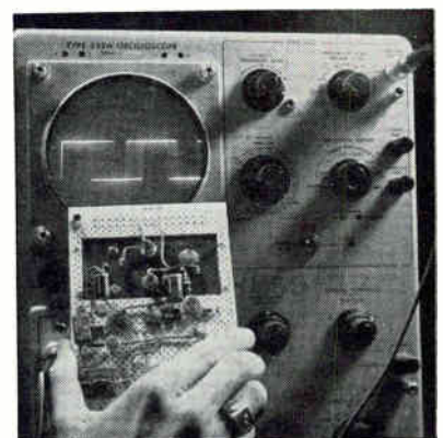
VERTICAL EDGES of signal train, as seen on scope, oscillate according to input voltage and frequency
