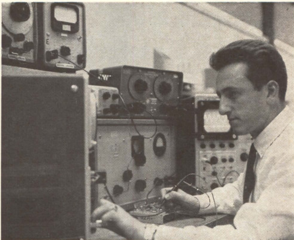
WIDEBAND AMPLIFIER is optimized for low noise with respect to both source impedance and input transistor
