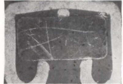
MICROSECTION shows wire being held onto post by spring action of terminal
