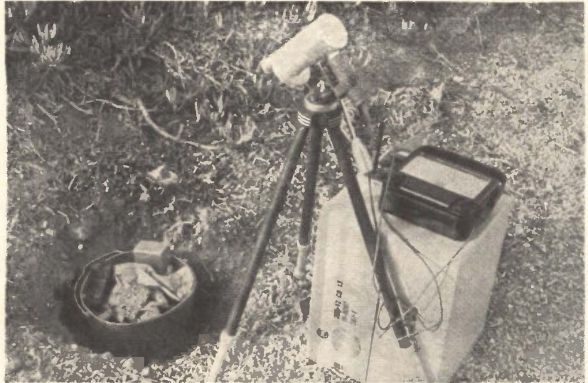
SIMULATED MINE was plastic bucket containing metal objects, fabric and fertilizer. Infrared detector, amplifier and readout meter shown at right—Fig. 1
