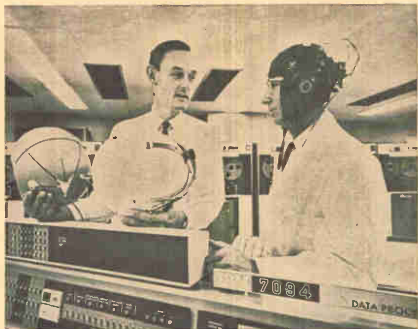
HELMET worn by scientist (right) at the University of California, Los Angeles, could take electroencephalogram readings from U. S. astronauts during extended space flights, UCLA says. Key element in the headgear is a microminiaturized preamplifier. Data is analyzed by an IBM 7094/1410 in UCLA's new computer center
