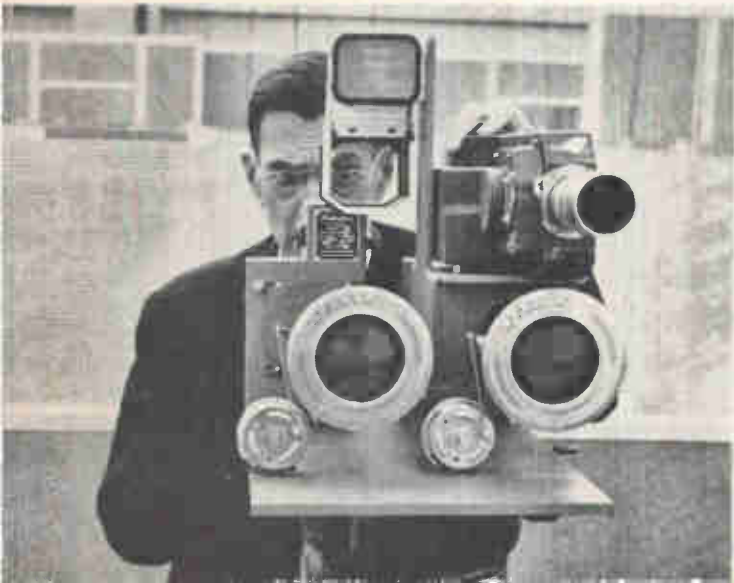
FLASH SPECTRA of the sun's corona were photographed during eclipse with this camera aboard the DC-8 by John Waddell of Douglas Aircraft
