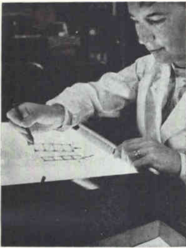
COMPOSITE electronic unit is made of 0.0005-in. thin Havar
