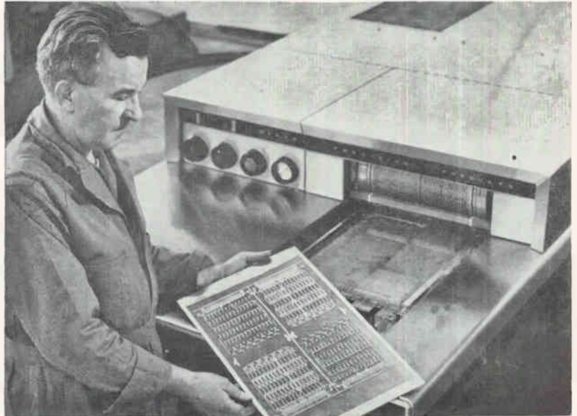
WHEN OPERATOR places copper-clad board and pushes a button, the machine produces printed circuit boards like one shown
