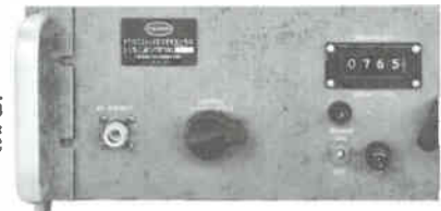
MODULAR SIGNAL SOURCE 1208 Freq. Range: 6.95 GC-11.0 GC
