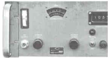
MODULAR SIGNAL GENERATOR 1108 Freq. Range: 6.95 GC-11.0 GC
