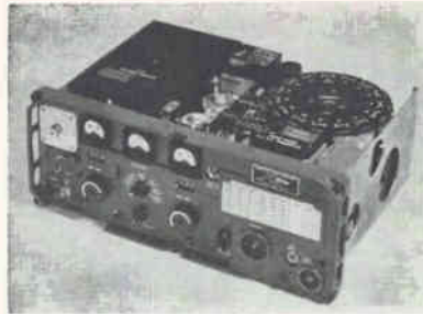
LINEAR amplifier portion of Army's new AN/GRC-106 ssb transceiver is typical of trend towards smaller high-power radios. This unit develops 400 watts
