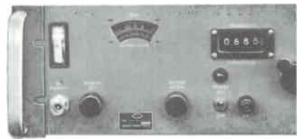
MODULAR SIGNAL GENERATOR 1107 Freq. Range: 3.8 GC-8.2 GC
