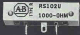
C HOT MOLDED ADJUSTABLE FIXED RESISTORS—Rated 1/4 watt at 70°C. Values to 2.5 meg. Tol: ± 10 and 20%.
