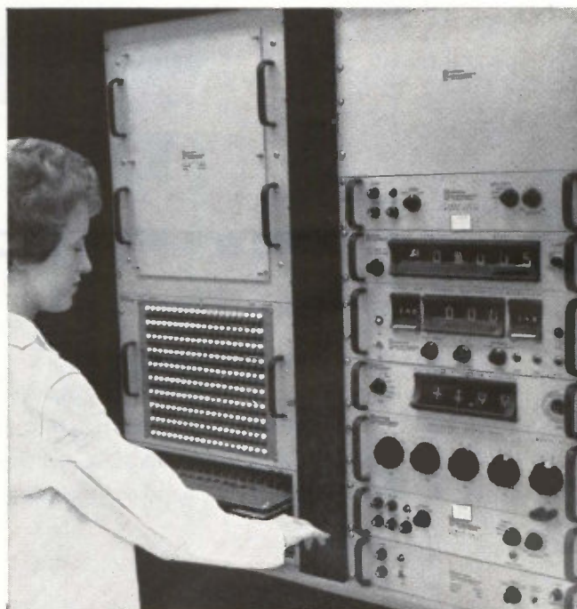
Technician at Electra Manufacturing Company inserts test resistors in the Automatic Resistor Data Logging System designed and built by Electro Instruments. Over 60 million resistor hours of data were accumulated in 18 months.
