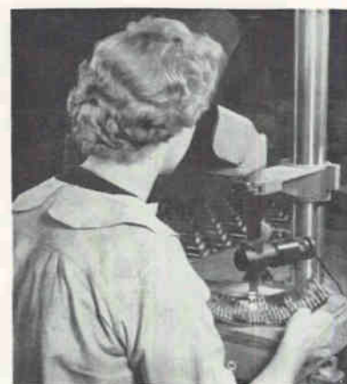
OPERATOR locates target holes in terminal board in platter fabrication section of Raytheon missile plant. Holes will then guide drilling of additional holes
