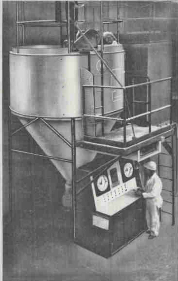
7'6" Dia. Nerco-Niro Packaged Spray Dryer
