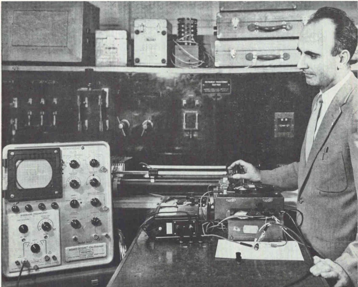
GATE TURN-OFF switch under test has the same physical configuration as a silicon-controlled rectifier
