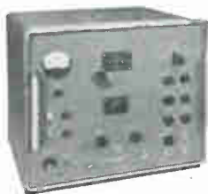
MODEL MSG-34 4.2 — 11.0 KMC. Accurately calibrated absolute power-level. Adjustable from 0 to -127 dbm from 1 MW.
