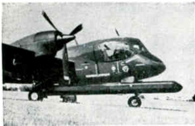
ARMY'S MOHAWK observation plane, outfitted with side-looking airborne radar (long pod below fuselage) for reconnaissance missions
