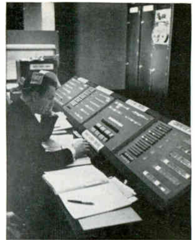
CONSOLE provides operating controls and selected readout
