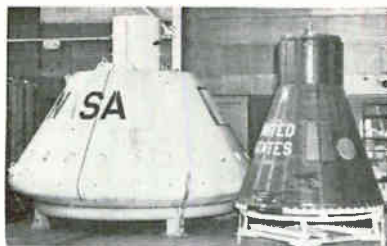
COMMAND MODULE of Apollo spacecraft will carry three men. Mercury capsule, at right, held one
