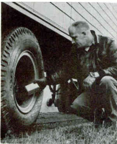
TRUCK DRIVER locates low tire with indicator by Magnavox. Indicator is used after transistor radio transmitters on wheels signal cab when pressure is low, as determined by valve pressure switch
