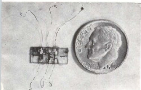
BLACK BARS are the three cryogenic bolometers that make up the radiation detector
