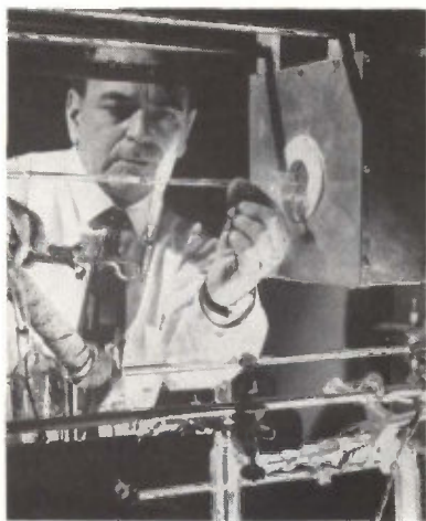
ABSORPTION CELL containing mercury isotope is sealed
