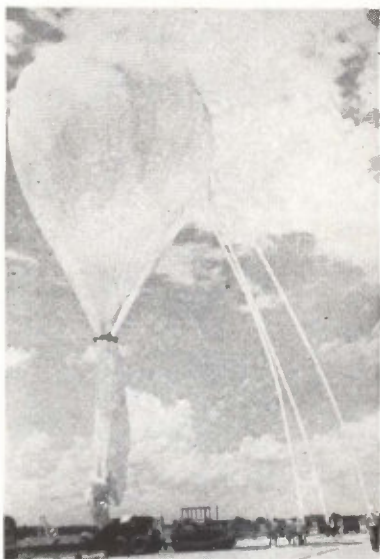
TEST LAUNCH of Stratoscope II flight system last year. Inflation takes 14,500 pounds of helium
