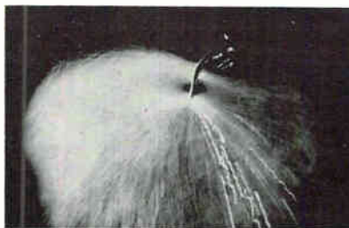
CAVITATION spray from a bent tip shows a clear nodal region of flexural motion—Fig. 2
