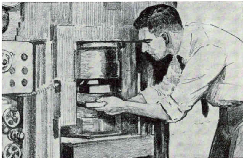
POWDERED COPPER is compressed at 50,000 psi into circuit-groove die prior to sintering in a reducing atmosphere. Rubber mat is used directly over circuit die
