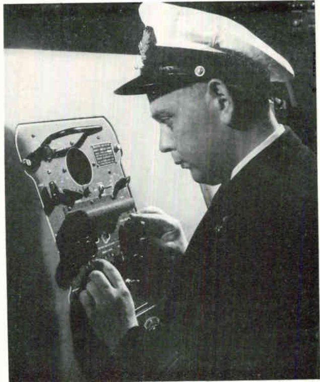
LORAN NAVIGATION equipment is favored by maritime operators. Position coordinates of ship at sea are obtained by officer using Sperry Gyroscope Co. receiver and world-wide loran network. Commercial loran C receivers are predicted
