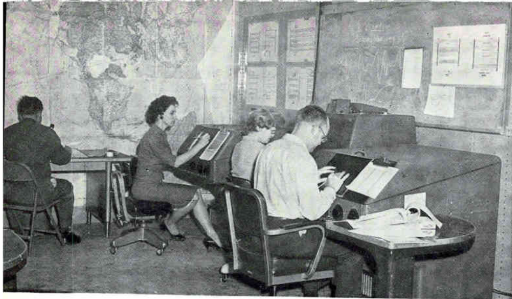
HIGH RESOLUTION , motorized film viewers for seismic analysis program compare two seismic signals. Digital and analog computers are also used in analysis
