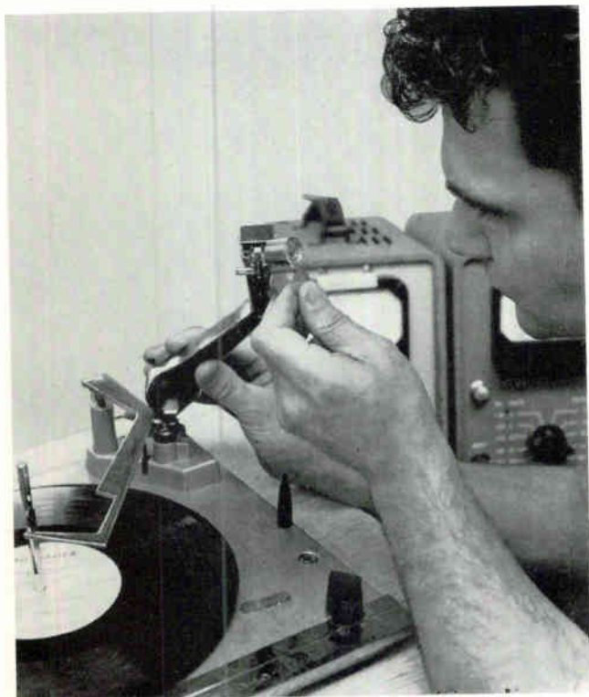
STEREO CARTRIDGE is examined under magnifying glass to assure correct seating of stylus, and positioning of diamond point in Motorola high fidelity instrument
