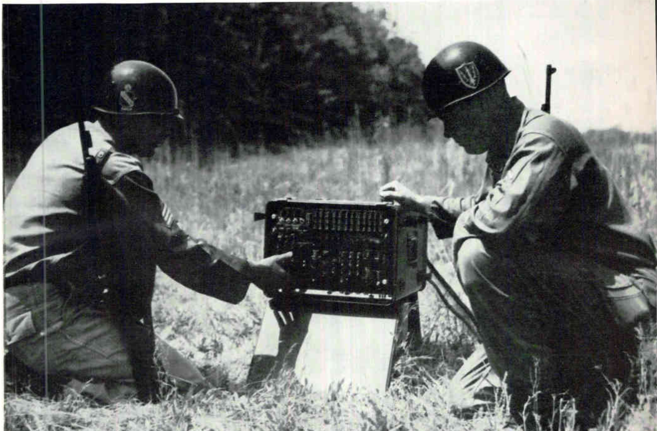
MICROPAC weighs in at only 90 pounds, but is a complete digital computer for tactical applications
