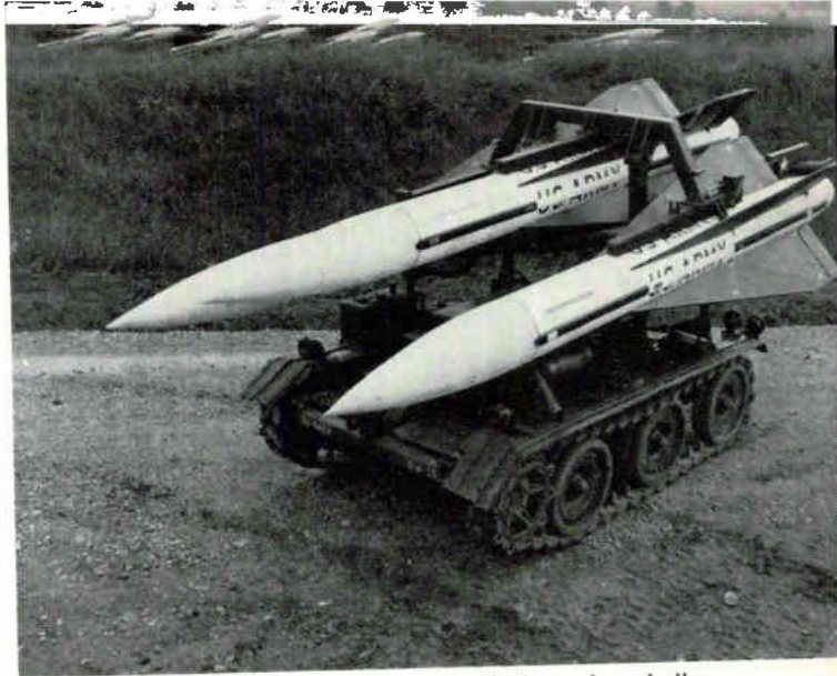
HAWK GUIDED MISSILES on mobile loader which carries missiles to launching site. Army's Hawk is built under Raytheon Company prime contract, is designed for surface-to-air-use
