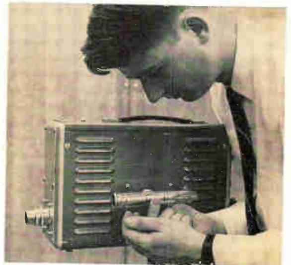
SLOW-SCAN VIDICON TUBE developed by Westinghouse Electric for use in tv systems operating at a rate of one picture every eight seconds. High resistivity photoconductive target is used
