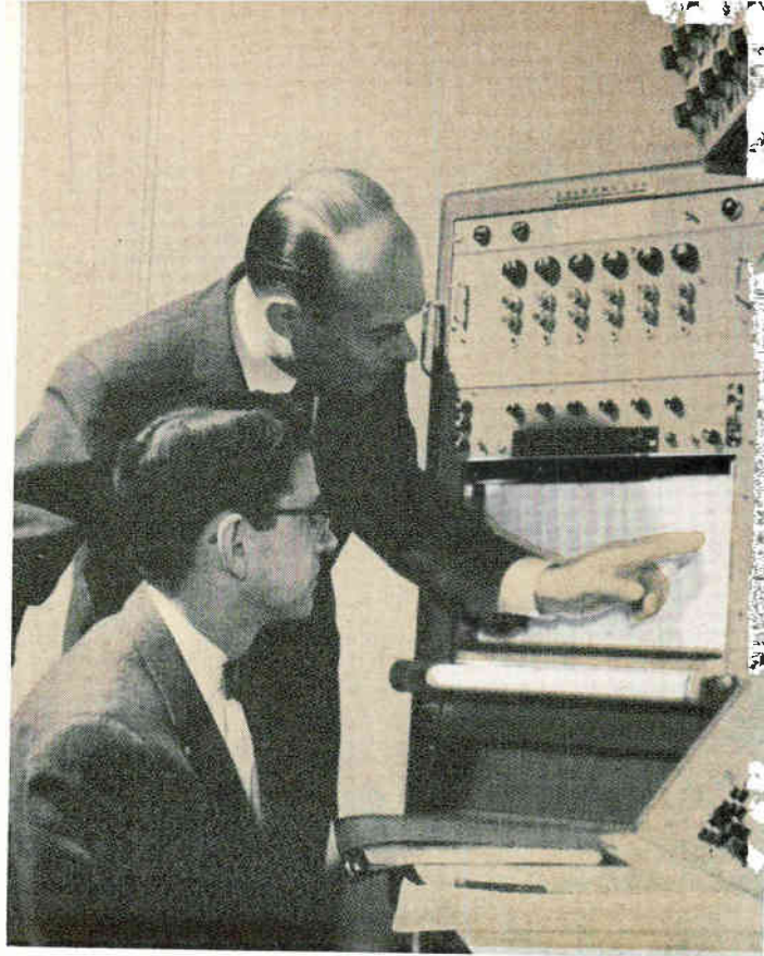
ANALOG COMPUTER in use to simulate a complete metal rolling metal in the mill, drives, regulators and control system on large
