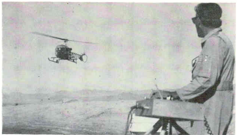
GROUND CONTROLS bring unmanned helicopter in for landing
