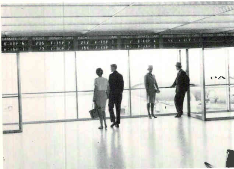
FLIGHT INFORMATION SYSTEM employing transistor operated control network is built in Switzerland. Tele-Norm Autophon equipment is shown at New York International Airport; similar systems are installed in European stock exchanges, industrial plants and banks
