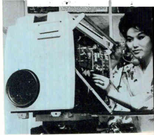
TRANSISTOR TV CAMERA built by Tokyo Shibaura Electric Co., Ltd. is designed for field or studio use. Instrument provides 525 line, 30 frame, scanning
