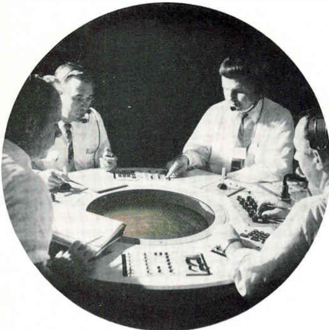
PLAN-POSITION DATA DISPLAY console built by General Precision Inc. is part of FAA's engineering model for testing new system design for air-traffic control. Direct-view storage tube is by Hughes Aircraft Co.
