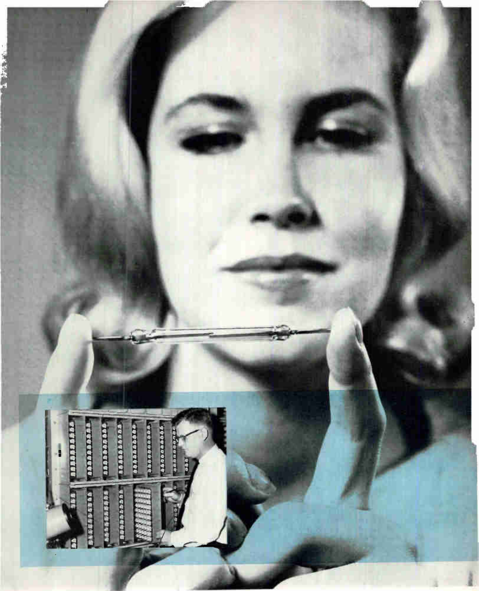
ELECTRONIC TELEPHONE EXCHANGE (inset), developed by Automatic Electric Co., a subsidiary of GT&E, is compatible with electro-mechanical switching equipment. Magnetic switches in hermetically sealed capsules (above) are used in switching matrix
