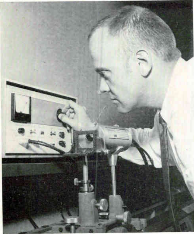
LASER WELDING promises to be one of the most fruitful applications of this new device. A Hughes Aircraft Company scientist prepares to fire a forced-air-cooled, ruby laser in a welding experiment
