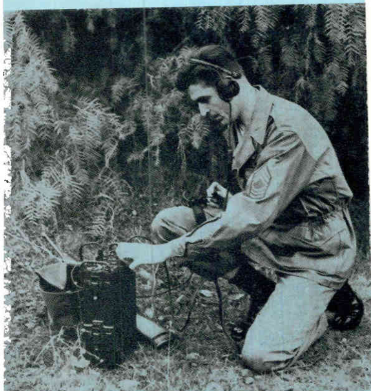
TRANSMITTER-RECEIVER undergoing field tests by U. S. Army. Built to provide dependable 300-mile range, the Sylvania Electric Products set has 10-watt power output, can be strapped to infantryman's back
