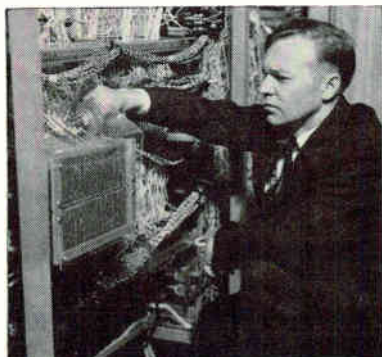
Magnetic core storages hold 4,096 26-bit words
