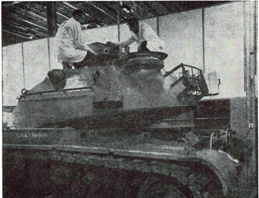
Minneapolis-Honeywell Ordnance Division engineers using SERVOSCOPE® servo system analyzer to make dynamic analyses of new gyroscope-stabilized tank gun-elevating and turret-traversing control system.
