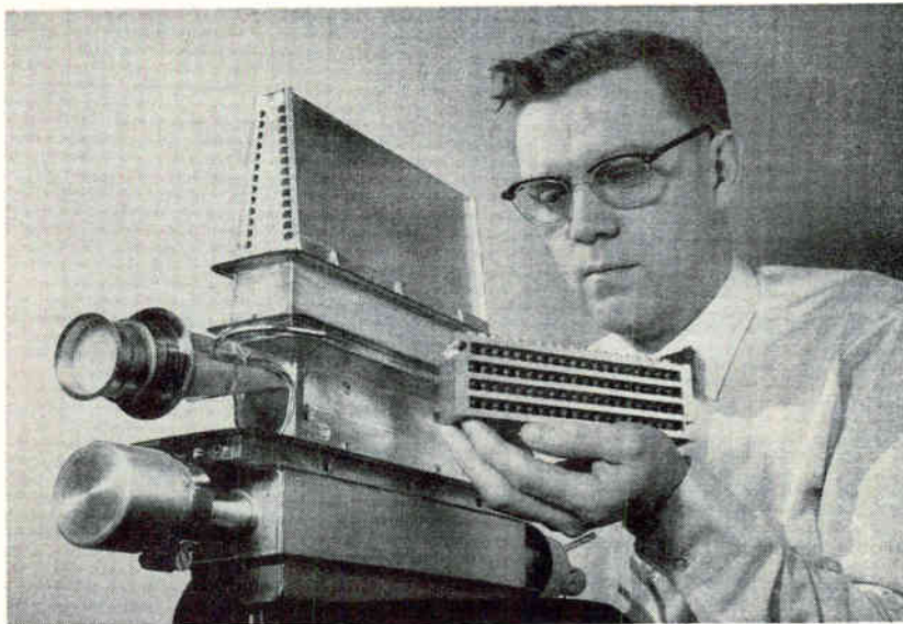
Multiple beam klystron by General Electric has single vacuum envelope, employs ten electron beams. Developmental model (above) operates at X band, produces C-W output of 32 kilowatts. Engineer holds multiple beam interaction section of tube
