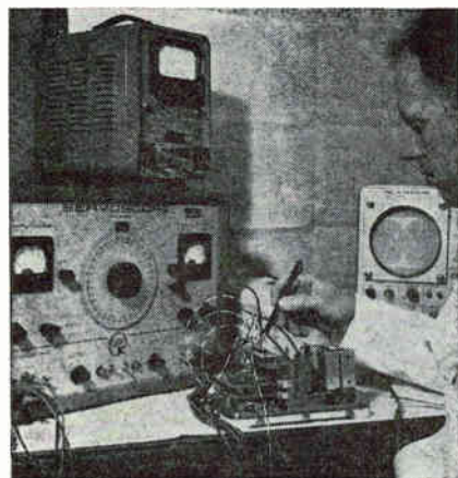
SERVOSCOPE® was also used in the development and testing of armored vehicle turret components. Engineer, above, is shown analyzing stabilizer current using SERVOSCOPE.
