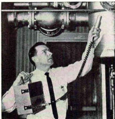
Delcon Corp., of Palo Alto, Calif., is making a battery-powered set which translates sound from the ultrasonic (35-45 Kc) to the audible range. It can be used to find leaks or flow obstructions in pressure or vacuum systems, or for engine analysis and other industrial applications
