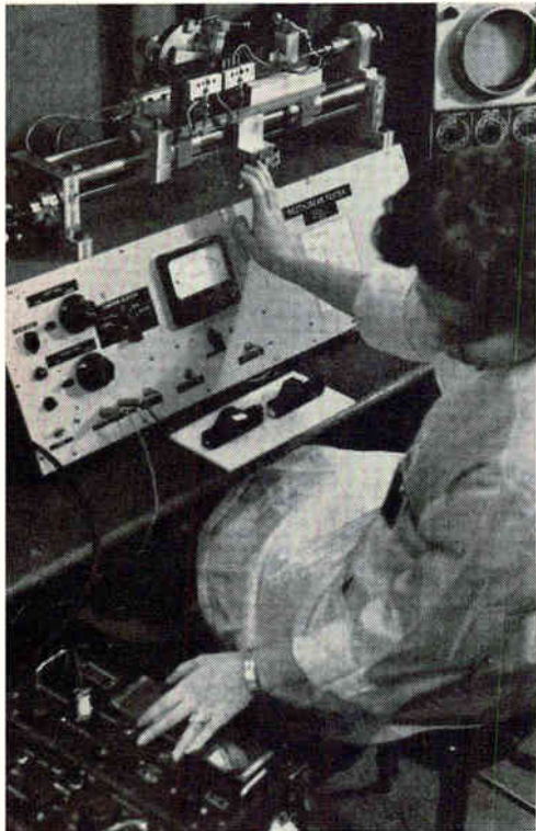
Linear drive mechanism tests potentiometers against 0.01 percent rotary master
