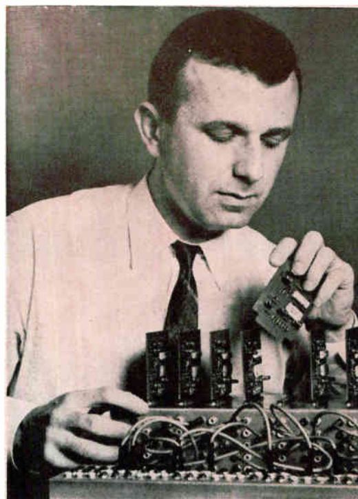
FIG. 5—Using assemblages of neuromimes, Harmon has demonstrated some functions of nerves in the eye and the ear
