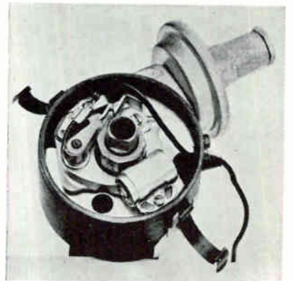
Distributor cam is replaced by toothed wheel that generates pulses in magnetic pickoff
