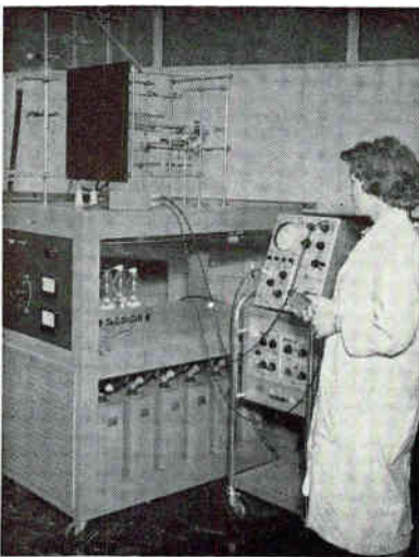
System for rapidly adjusting film resistors could be used to adjust resistances in microcircuit films and in composite printed circuits
