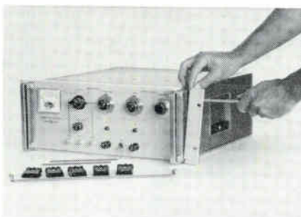
Bench model instruments in the new modular form factor are rack mounted merely by removing the feet and attaching two brackets furnished. Shown: Model 716A Klystron Power Supply.
