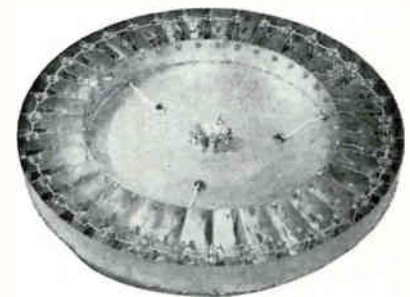
Bottom view of wave antenna switching unit
