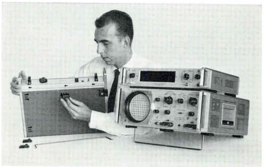
Bench model instruments in the new modular form factor are rack mounted merely by removing the feet and attaching two brackets furnished. Shown: Model 716A Klystron Power Supply.
