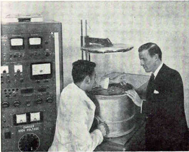
Resistors and capacitors are deposited on 20 substrates at a time in high-vacuum chamber
