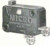
Screw terminals. SP-NO. 15 amps.
