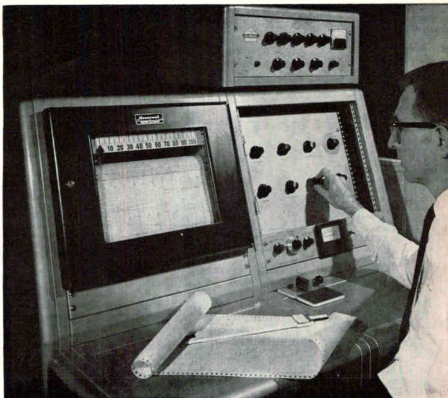
Research chemist investigates moisture content of living tissue using Schlumberger's model 106 nuclear magnetic resonance analyzer
