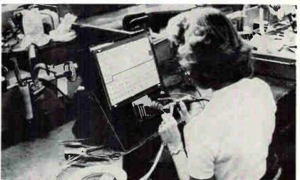
Panel helps locate pins of plugs by lights in panel. To wire a given plug, the operator selects a plug adaptor and chart to match the plug. When operator touches the soldering iron or probe to a plug pin, the corresponding number or letter lights up on the chart. The panel can also be used as a fixture for plug inspection. Panel was developed by Winslow Product Engineering Corp., Arcadia, Calif.
