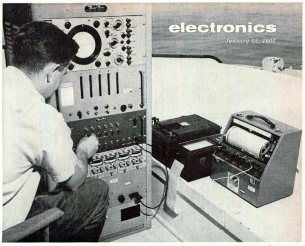
FIG. 1—Information transmitted to the receiving station aboard boat is checked by sonar technician. A probe is lowered to 2,000 feet and water temperature and pressure data telemetered
