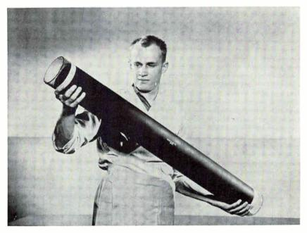
GLASS RESISTORS four feet long serve as dummy antenna loads for testing and calibrating transmitters and as power dissipating terminations for rhombic and other transmitting antennas.
