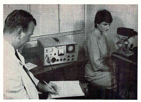
Flicker-fusion tester in use. Ammeter indicates light brightness, cathoderay tube presents ratio of on and off times
