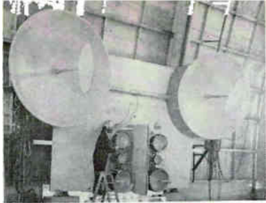
TRANSMITTING and receiving antennas of the four-band radar system are separated for bistatic studies
