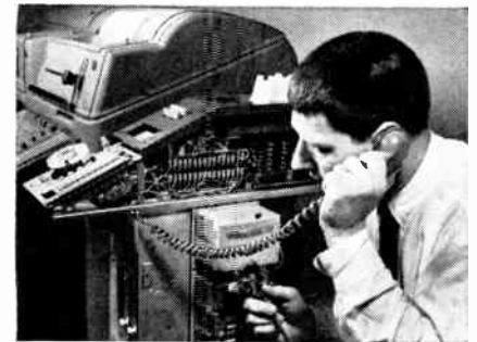
New York Laboratory, N. Y. We were studying the performance of a new data set which converts teletypewriter pulses into tones for transmission over regular voice circuits. Transmitting teletypewriter messages over voice circuits was introduced on August 31, 1962.
