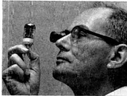
Allentown Laboratory, Pa. We were working with engineers of Western Electric, manufacturing unit of the Bell System, on the manufacture of long-life electron tubes for a new deep sea cable system.
