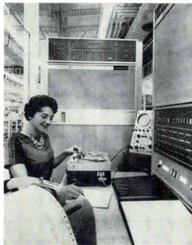
TO SIMULATE transmission lines and remote equipment, simple tape recorder is used
