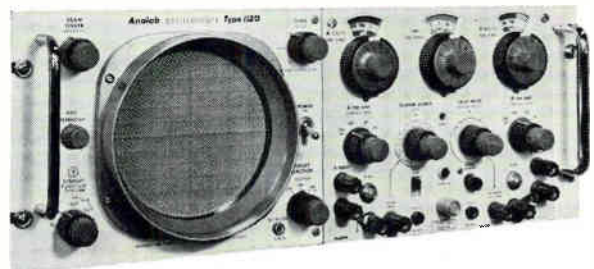
One of 46 Analab Type 1120R/700 scopes being used at Avco. 100 \mu /cm sensitivity and direct-reading null-readout dials permit measurements of amplitude, time, and phase to \pm 2\% accuracy.
