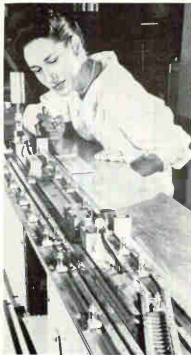
ASSEMBLY fixtures with tube structures move on conveyor from automatic assembly station
