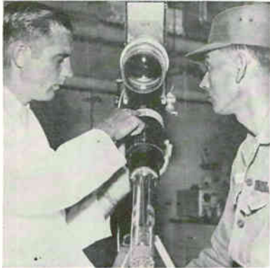
INTENSIFIER tube couples to standard tv orthicon tube to televise night operations. It intensifies images some 80,000 times
