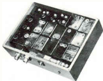
Developmental model of 400 MC transponder, utilizing welded module construction
