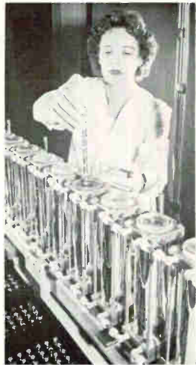
NUVISTORS are being loaded into vacuum baking and sealing chamber
