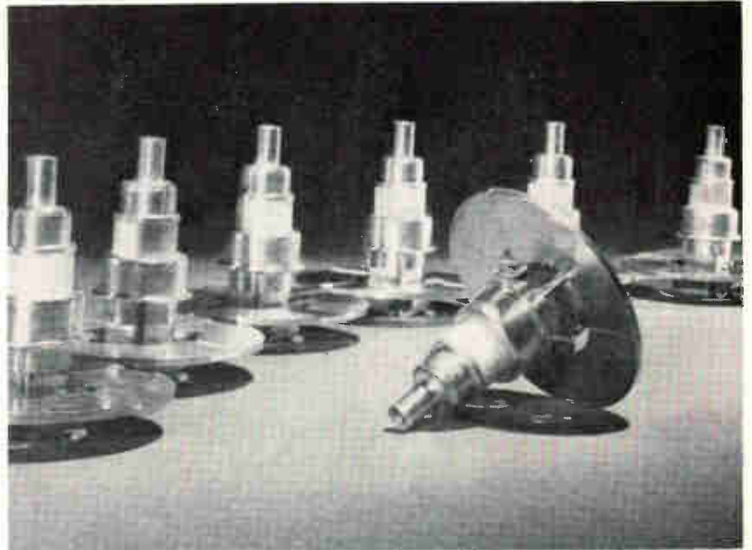
LIGHTHOUSE tubes designed for continuous operation in communications satellite transponders. Large disk serves as heat sink
