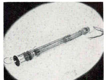
BACKWARD-WAVE converter developed by ITT is an electronically swept receiver in glass envelope (right). Proposed version (sketch) would have built-in i-f amplifier and may be used in millimeter-wave region
