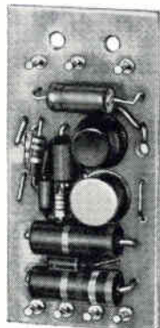
"DC Pulse Circuit" produces square wave millisecond pulse for high speed devices. Data Sheet 194.
