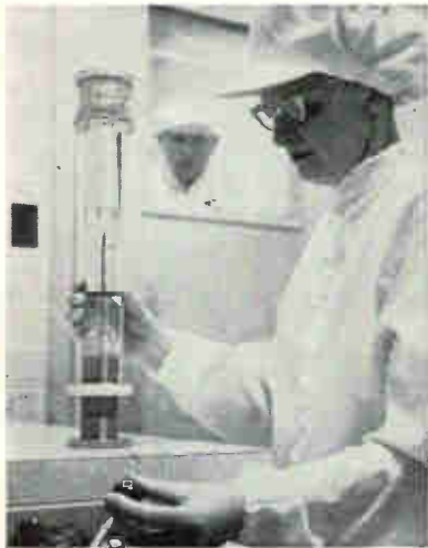
OPERATING the lever causes fluid to drive elevator up until target mounting ring snaps in place
