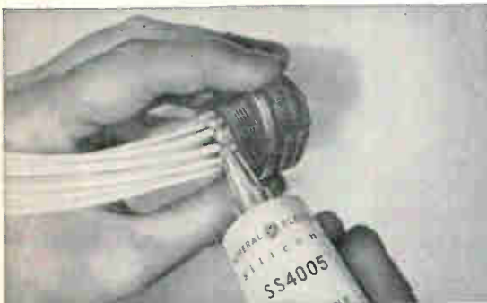
CORROSION INHIBITORS Silicone compounds protect against sticking, moisture, corrosive atmosphere.
