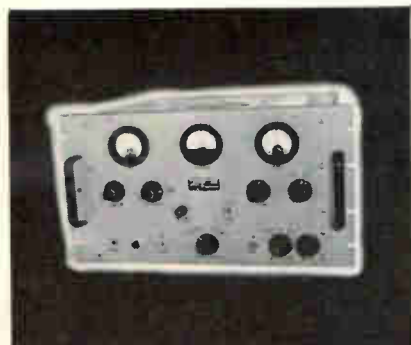
1700-MC Special-Purpose Ground Checkout Receiver Type 49A1. One of a series from 900 MC to 2400 MC.
