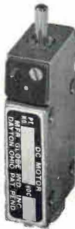
TYPE VS 7/16" flat .0025 hp @ 8,000-17,000 rpm.
