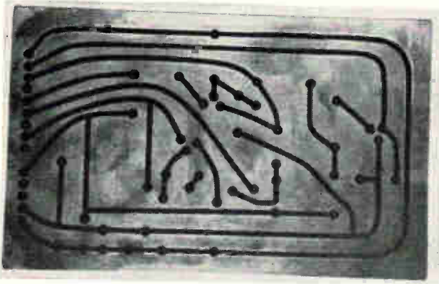
TYPICAL p-c board, ready for etching, left, and etched board with connector plug and copper eyelets added. Using p-c boards in prototype circuits has advantages where stray capacitance and crosstalk effects may influence final circuit
