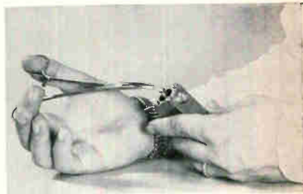
TUNNEL DIODE is inserted in oscillator mount
