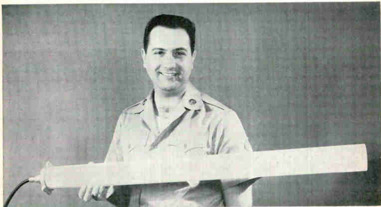
EXPERIMENTAL ANTENNA using a glass fiber tube is light and rugged
