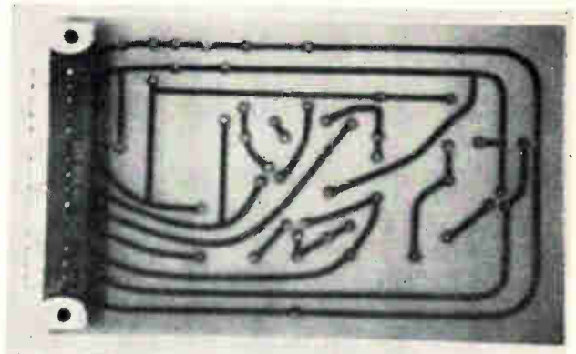
TYPICAL p-c board, ready for etching, left, and etched board with connector plug and copper eyelets added. Using p-c boards in prototype circuits has advantages where stray capacitance and crosstalk effects may influence final circuit
