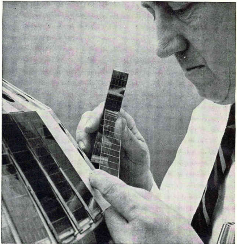
SOLAR CELLS and transparent sapphires are being attached to a developmental model of Telstar communications satellite by Bell Labs engineer
