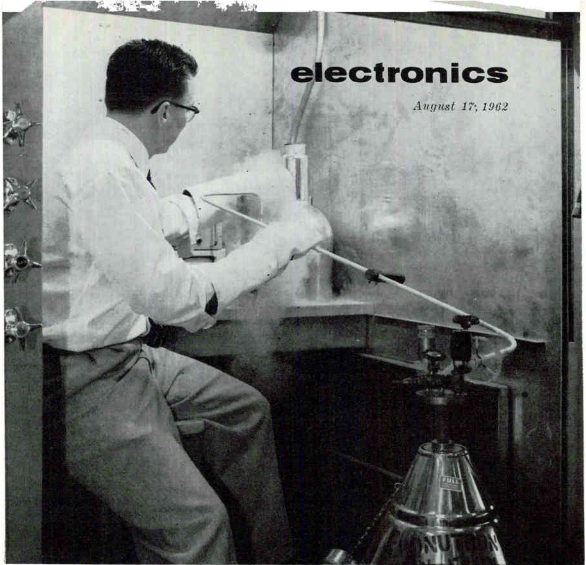
AUTHOR Lambert filling a nitrogen jacketed cryostat with nitrogen
