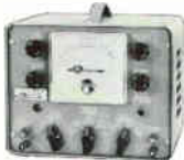
Pulse Meter Furnishes a convenient method of measuring dial speed and percent make.
