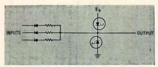
LOGIC CIRCUIT, heart of digital differential analyzer, uses two tunnel diodes with valley switching—Fig. 1
