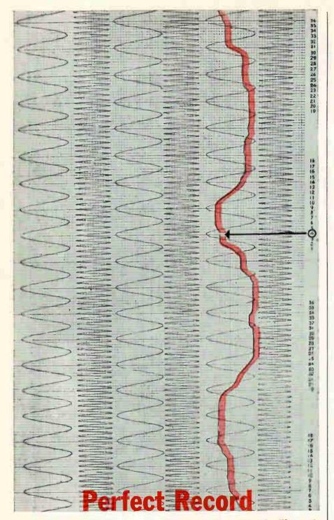
CEC's Type 5-123 Multi-channel, Direct-print Recording Oscillograph gives you: complete front access; twelve discrete speeds from 0.1 to
