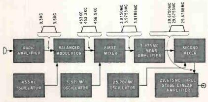
SSB EXCITER for upper sideband frequency synthesis-Fig. 1
