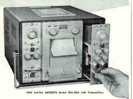
Measures and records virtually everything... anywhere... strain, temperature, displacement, force, flow, proximity, depth, pressure, electrical, chemical, radiation, etc.
