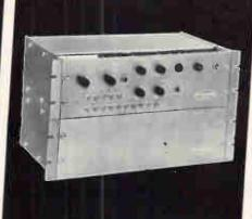
**ELECTRONIC COMMUTATOR** combines the advantages of both mechanical and electronic commutators...Scanning rate up to 1000 data points per second and 12 levels per cross point permits simultaneous scanning of differential inputs, shields of balance lines, calibration circuits and associated data.
