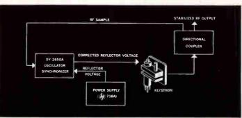
The DY-2650A is essentially a crystal-controlled superheterodyne receiver terminating in a phase comparator. An oscillator sample is mixed with harmonics of the rf reference to produce an intermediate frequency of 30 MC, which is compared in phase with the 30 MC reference. For stabilizing a klystron, the resultant phase error voltage is added in series with the klystron reflector power supply voltage.
