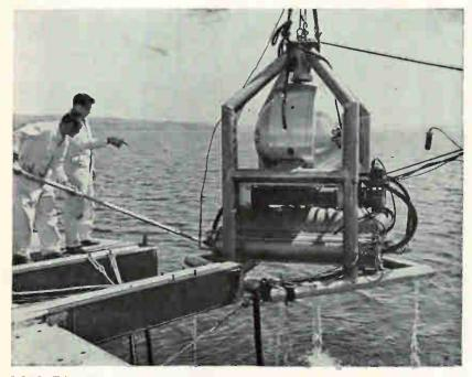
HIGH-POWER, LOW-FREQUENCY sound generator, shown under test at lake, was designed by General Dynamics/Electronics for Navy antisubmarine-warfare studies. A pump-driven valve amplifier converts a fluid flow to vibratory energy, driving two aluminum hemispherical pistons (seen below apex of frame). An electronic oscillator is used for control
