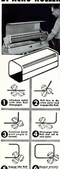
Forming small and large circles without flat spots and a variety of other sheet metal shapes is easily accomplished on the Di-Acro Roller with its exclusive cam actuated Idler Roll. Rear roll indicators allow operator to quickly return to a previous setting. Eight models from 6" to 42" forming width.
