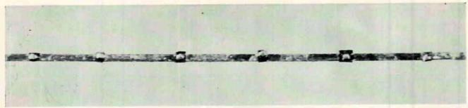
THIN GLASS chain links many silicon diodes. Use for designing memory plane does not require redesign of circuits
