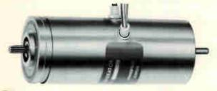
NEW FEATURE ADDED TO SIZE 10 and 11 MOTOR GENERATORS Sangamo's standard size 10 (.938" dia.) and size 11 (1.062" dia.) servo motor generators are now available with a rear shaft extension to permit mechanical coupling and/or speed checks after the unit is installed. Positive alignment is assured by the use of three ball bearings in each unit.
