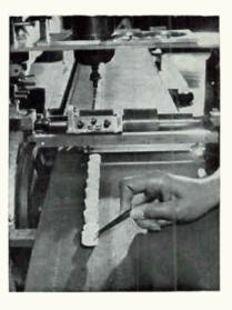
METALIZING COATING is applied automatically by rollers to ends of ceramic cylinders. The cylinders will be heated in a six-stage hydrogen furnace to fuse the coating to the ceramic
