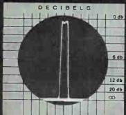
This extremely accurate log amplifier enables exact measurements of attenuation in networks, filters, amplifiers, and other devices exhibiting dynamic operating ranges down to 90 db. Total rf response of device under test can be displayed in a precise logarithmic ratio on a standard dc-coupled oscilloscope. Write for complete technical data.
