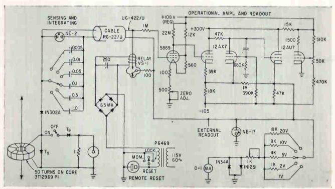
INTEGRATING AMMETER has the range switch at the pickup for maximum convenience. If a commercial electrometer is used, only the sensing and integrating portions of this circuit are needed—Fig. 2
