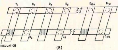
MEMORY PLANE schematic (A) of diode core. Construction (B) with diode ribbon strips shows how factory-welded matrix replaces 192 individual diodes
