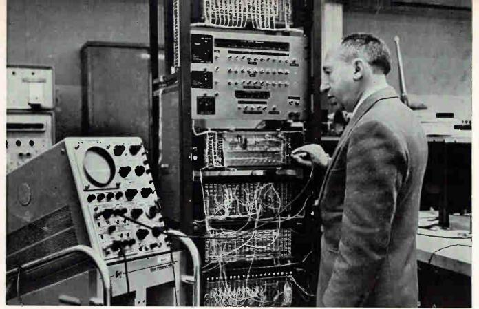
DIGITAL-ANALOG CONVERTER. Author measures a d-c level output from converter
