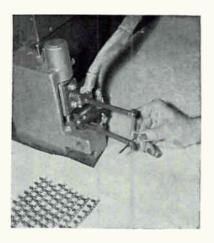
CONTACT CONTAMINATION is one of the major causes of trouble in relays and choppers, and a major source of contamination is the solder flax used for making internal connections and sealing the cans. Cambridge Scientific Industries, Cambridge, Md., has therefore turned to spot welding for internal connections in their choppers and to heliarc welding for sealing the can.
