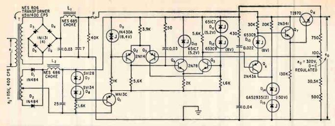
REFERENCE POWER SUPPLY relies on a temperature-compensated silicon junction zener diode as the basic reference element with precision wire-wound resistor network to obtain error signal—Fig. 2
