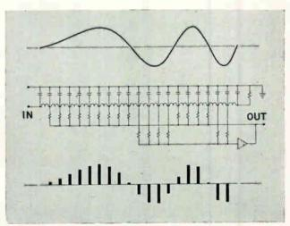
RESISTOR MESH used for generating a chirp signal—Fig. 3
