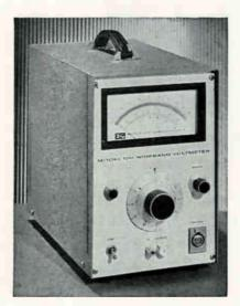
taneous viewing during measurements. When used as a wideband preamplifier, output impedance is 50 ohms with a rise time of less than 6 ns. Gain stability is assured by over 100 db of negative feedback. There is a complete absence of low-frequency jitter either due to amplifier noise or line transients. Change of range is by interstage attenuator.
