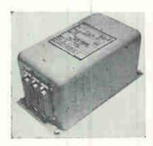
Stepping Switch Controls 468 Circuits
