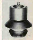
NEW FLAT PACK (left center is being used by Minneapolis-Honeywell for 65-amp transistors. Eimac is showing vapor-cooled high-power tetrodes (right)
