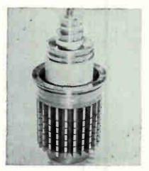
Vapor-Cooled Triode Has High Power Level
