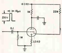
ators, and have been used as high energy film markers, photomultipliers and shunting devices. The sketch shows typical operation in a trigger circuit. (302)
