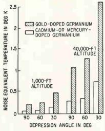
Noise equivalent temperature of cadmium- or mercury-doped germanium is several times that of gold-doped germanium-Fig. 2
