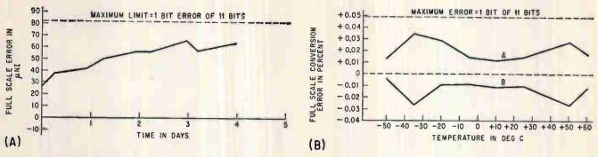
FULL-SCALE conversion error variation with time (A) and full-scale conversion error versus temperature for 11-bit current decoder (B)—Fig. 4
