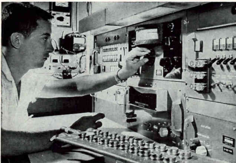
MANUFACTURE of power transistors with a reliability of 99.997 percent is claimed by Delco Radio, under R&D contract with Autonetics, Minuteman guidance contractor. Test set shown checks out eight parameters of a transistor in eight seconds and records results on punched cards. Transistors are checked in 20-unit racks
