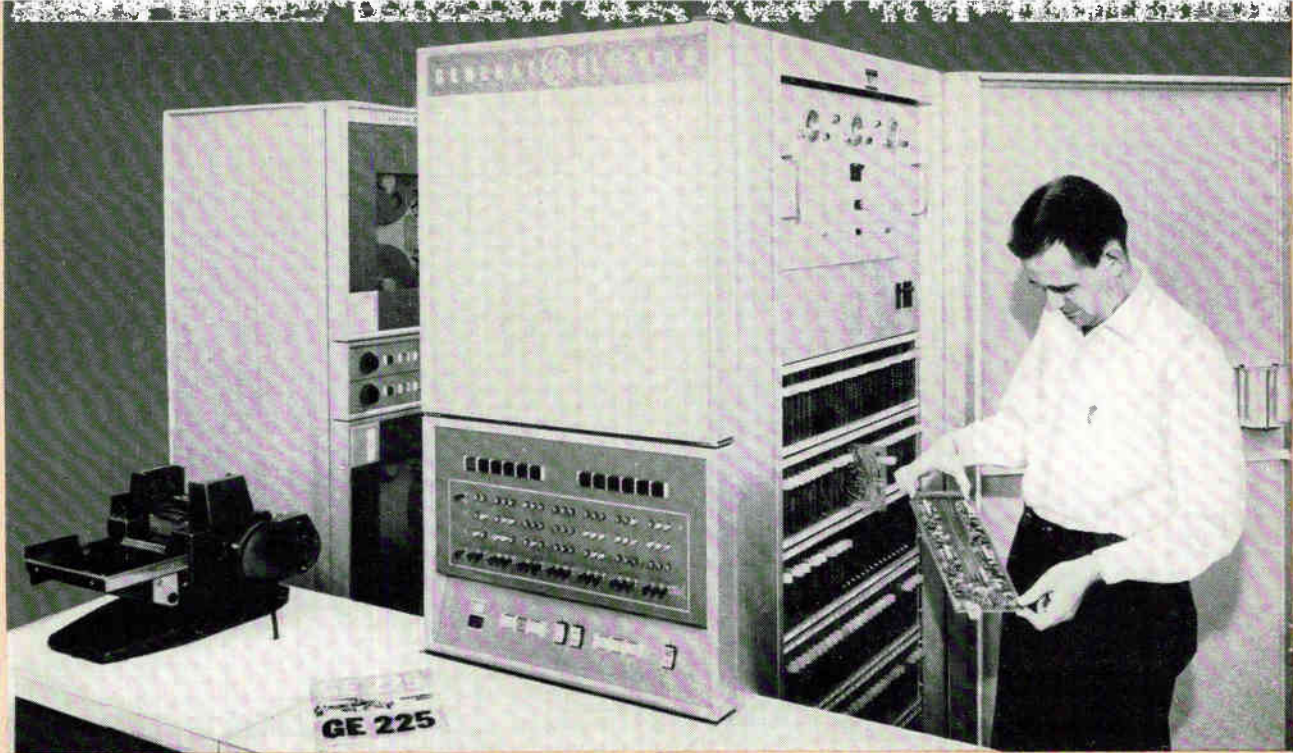
Engineer examines one of 750 printed-circuit, logic-component pluggable cards in GE 225 computer at Western Reserve University's Center for Documentation and Communications Research. Each reel of magnetic tape in upper left of console stores the equivalent of approximately 2,500 documents
