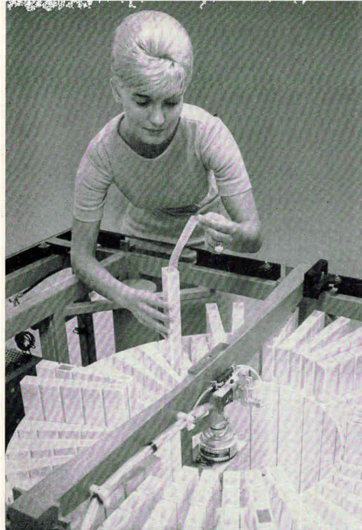
Each bin, or document file, of IBM's Walnut system contains 200 plastic cells loaded with film strips containing images equivalent to about 3,000 average-sized books
