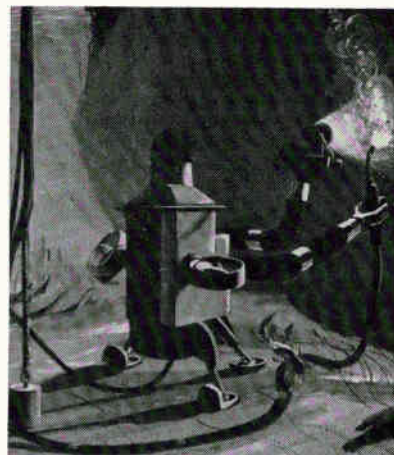
UNDERWATER MOBOT , as the artist visualizes it at work. System is a variation of one used on land for nuclear handling
