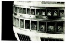
Section of satellite shows equatorial antenna slots. Upper row transmits, lower row receives microwave signals.
