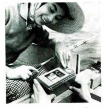
Nippon Electric calls this gadget a fish camera, It's a transistor sonar set. Frequency is 200 Ke, maximum depth 200 feet, price in Tokyo \$110
