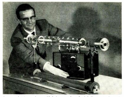
Output of 1.5 mw is provided from each end of helium-ncon laser introduced by Raytheon and warranted for 1,000 hours continuous operation
