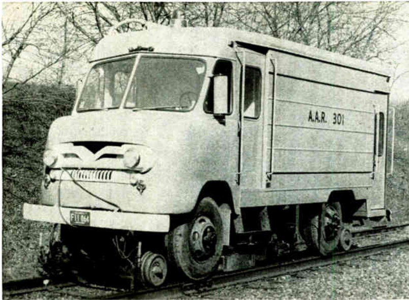
Road-rail trucks generally carry 12 amplifiers to obtain data on rail condition
