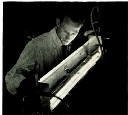
Helium lamp source is r-f powered
