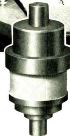
ZP-1025 (shown 2 3/8" actual size) reflects design trend in G-E IFF tubes.
