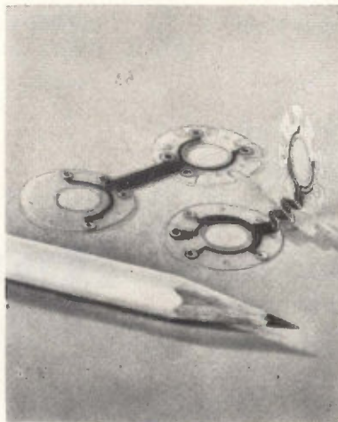
Flexible etched cable used in aircraft instrumentation improves reliability, saves space and weight
