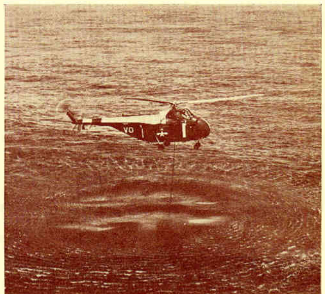
Navy helicopter searches for submarines with sonar dome lowered into sea. Transducer may be lowered below sound bending thermal layers that would allow undersea craft to remain undetected
