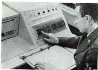
Information from human observers can be fed manually into automatic weather station
