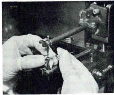
A spot of foreign matter on a lead will usually cause a bad weld
