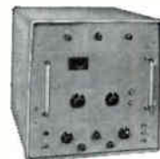
Model CSG SWEEP GENERATOR 1,000 to 16,000 mc In 5 interchangeable tuning units
