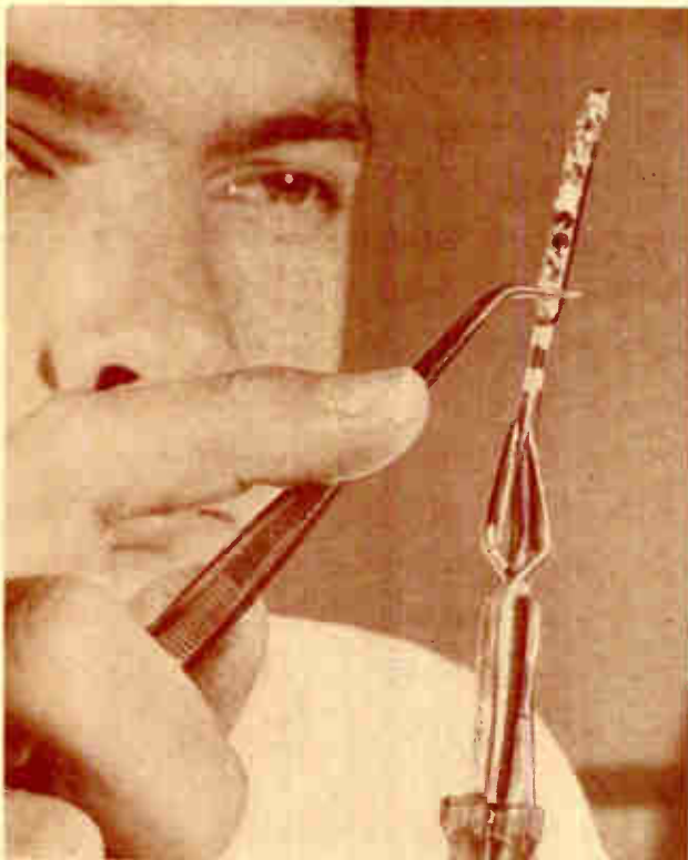
Medical probe contains radiation detector and microminiaturized electronics. Hughes Aircraft unit placed in 3-mm catheter can be inserted into human vein to measure radioactive isotopes in the blood stream
