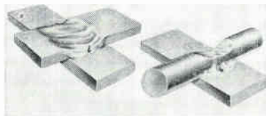
Blow holes or deep pits cause weakness. Blow holes can develop if the electrode force is removed before the weld is actually made, if the material is dirty or contains a large amount of impurities
