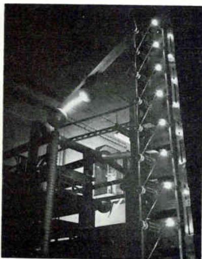
Lightning-like bolts test klystron tubes used in radar. Sperry facility can deliver 100 million watts of peak power
