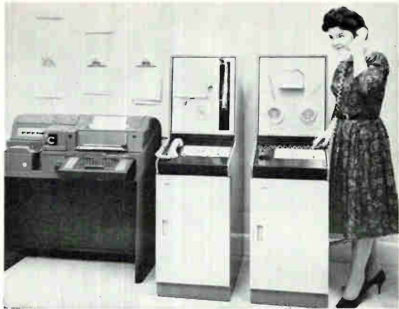
Dataspeed, high-speed paper tape transmission system by AT&T, sends 750 bits a second over regular telephone lines. Photo shows teletypewriter with tape reader and punch attachments (left), Dataspeed tape punch or receiver (center), and tape reader or transmitter
