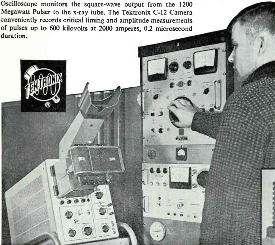
Adjusting for impedance match of T-F emission tube to square-wave pulse of new x-ray system manufactured by FIELD EMISSION CORPORATION, McMinnville, Oregon.
