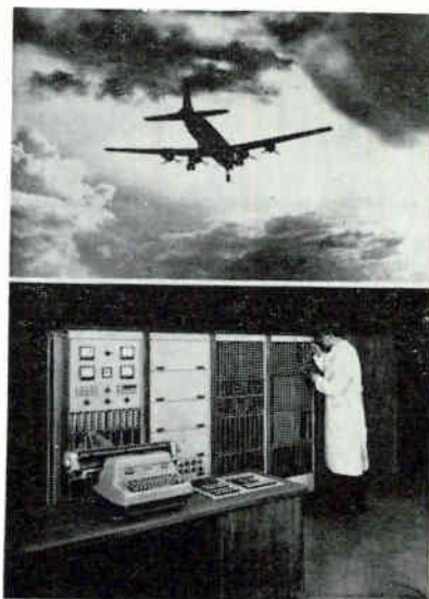
German air traffic control digital computer TR4 (Telefunken) is part of new system installed in Frankfurt
