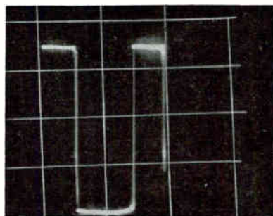
FIG. 3—Waveshape: V_1 = 3.6 v d-c, f = 71 cps, C_3 = 0.3 \mu\text{f} and R_3 = 150,000 ohms
