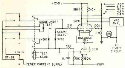
FIG. 3—Typical test circuit uses difference amplifier to trigger magnetic amplifier to signal reject
