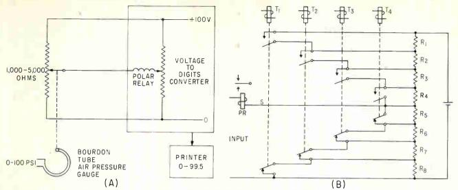
FIG. 1—Digital air-pressure recording system (A), with converter shown in simplified form. In an elaboration of the basic system (B) the T relays operate in combinations to i clude or short out various resistances in the voltage divider chain. For example, if relays  $T_1$  and  $T_2$  are operated, resistances  $R_1$ ,  $R_2$ ,  $R_3$  and  $R_4$  are shorted out, and the others remain in the circuit. The converter uses 9 T relays and 18 divider resistors
