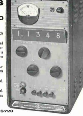
INPUT IMPEDANCE: 2 megohms in parallel with 15 pF to 45 pF
