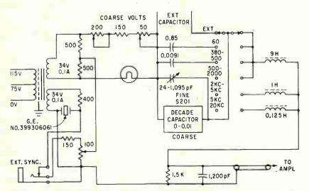
FIG. 4-Details of thermal bridge and filter for use from 50 cps to 2 Kc
