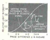
Fig. 2-Relationship between optical phase retardation and intensity of light reaching the multiplier phototube
