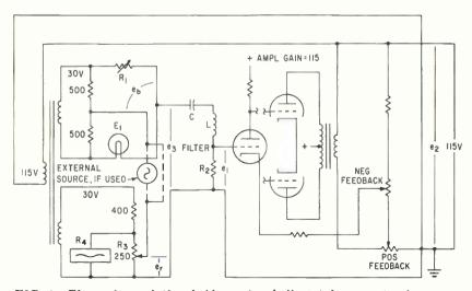
FIG. 1—Thermal regulating bridge using ballast tube operates in power oscillator to maintain output voltage constant
