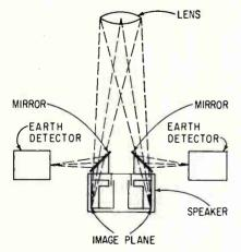
FIG. 1—Relative pulse durations from oppositely located indium antimonide detectors depend on earth's position with respect to optical axis
