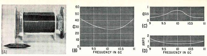
FIG. 4—Tetrahedral junction switch (A) from Caswell Electronics. When nonenergized, insertion loss is high at all points of the normal waveguide operating band (B); minimum insertion loss with current optimized (C); and current required to minimize insertion loss (D). In this switch, energy not transmitted is reflected rather than absorbed
