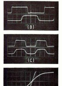
Block diagram of delay measurement system (A). Waveforms show input and output voltage steps of delay line, at a low repetition rate (B), approximate coincidence (C), and exact coincidence (D), with horizontal scales of 0.2, 0.1, and 0.014 µsec per cm, respectively
