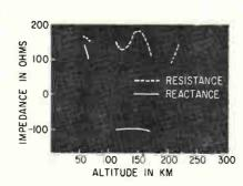
FIG. 8—Antenna impedance curves at 7.2 Mc (curves are shown where conditions permitted data reduction)
