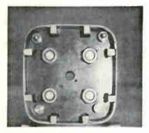
Parts located in welding fixture (top view)
