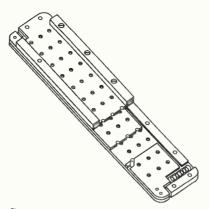
Cutaway sketch of pellet loader. Holes in the three plates line up when fixture is squeezed
