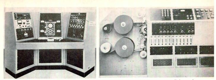
Manual diode tester (left) checks 1,200 diodes per day while automatic tester (right) checks up to 18,000 diodes per day
