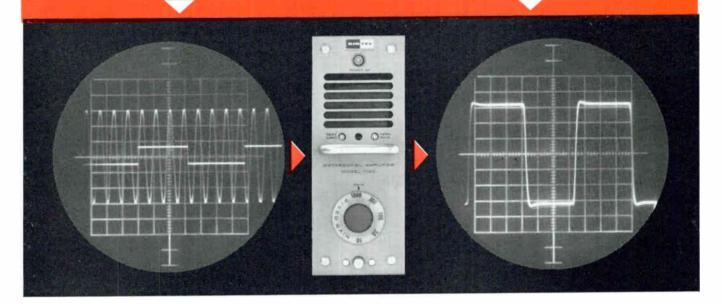
If you measure the output of thermocouples, and the thermocouples are bonded to a rocket engine or almost any other grounded object, and the distance between thermocouples and amplifiers is more than a few feet, you should consider the above illustration carefully. While we'll admit your thermocouples probably aren't producing square waves, nine chances out of ten you do have a problem with 60-cycle common-mode noise. Nearly everybody does.
