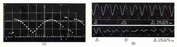
FIG. 5—Typical telemetry record (A) using automatic decommutation; and standing-wave patterns (B) taken on Aerobee rocket S/N-37 White Sands Missile Range, New Mexico, August 28, 1959 (automatic decommutation system not used): left record is with 3-Mc antenna, right with 7.2-Mc antenna
