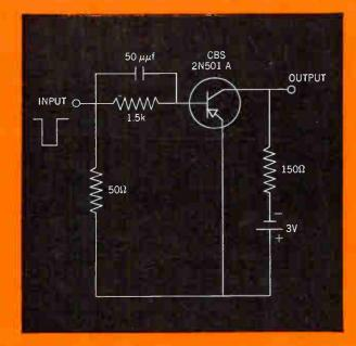
**IN THIS NEW CIRCUIT,** CBS 2N501 and 2N501A transistors achieve delay, rise, storage and fall times of 2.0, 3.7, 3.2, and 2.3 ns respectively.
