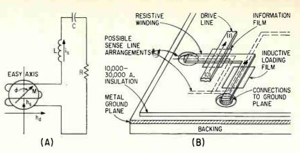
FIG. 2—With proper film and circuit parameters, this circuit (A) may be used as a flip-flop in which the magnetization M in the film is switched from either one of its rest orientations to the other by successive drive field pulses,  $h_4$ . Reliability of magnetic-film memory can be increased by passive R-L loading (B)
