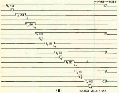
FIG. 2—The partial schematic (A) shows the first two of the nine sets of relays in the converter. The combination of locked T relays in the comparison sequence (B) determines the voltage value to be printed out
