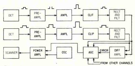
FIG. 2—Unequal length pulses from each detector of pair are converted to d-c voltages and applied to differential amplifier to produce off-axis error signal
