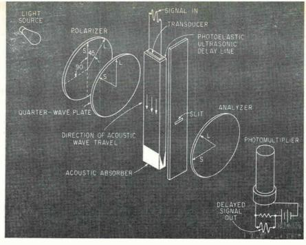
Fig. 1—Schematic arrangement for reading out the acoustic wave data as it passes down the glass delay line
