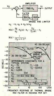
FIG. 3—Transfer function and frequency response
