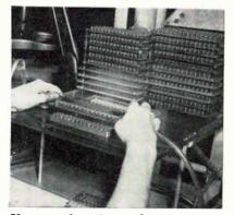
Vacuum bar is used to pick up pistons and drop them in boat
