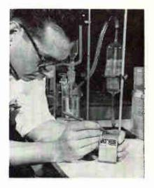
A RECHARGEABLE nickel-cadmium battery with a true hermetic seal, specifically designed for high reliability, long-life outer space performance was revealed by Gulton Industries, Inc., of Metuchen, N. J.
