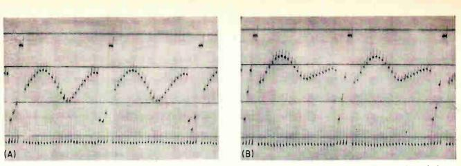
FIG. 7—Record at 7.2 Mc (Acrobee 150 IGC No. AA3.183C) : normal standing wave (A) taken at 65 seconds, and abnormal standing wave (B) taken two seconds later. Fig. 8 shows corresponding impedance changes
