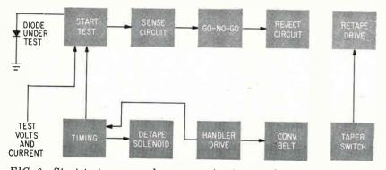
FIG. 2—Start test, sense and go no-go circuits are elements of a typical test pack. Remainder of circuits are used in all tests
