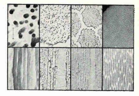
MAGNETICS. These are micrographs of longitudinal (bottom) and cross section of iron wires in a copper alloy matrix made by wire drawing. This technique is used to prepare elongated iron particles with diameters less than 1,000 angstroms. Work was recently described by F. E. Luborsky of General Electric Research Laboratory at the Sixth Annual Conference on Magnetism and Magnetic Material<sub>3</sub>. For other conference highlights, see Assistant Editor Lindgren's article (p 81).
