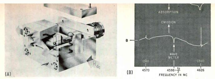
FIG. 3—Developmental design of ferromagnetic parametric amplifier (A), and the effect of longitudinal pumping on a pair of magnetostatic modes (B). Curve A is without pumping; curve B is with pumping
