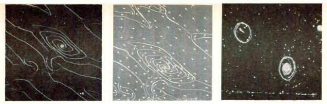
FIG. 6-Powder patterns of spiral walls in thin magnetic films, left, consist of a pair of antiparallel domains wrapped about a central point through many revolutions. Ellipticity results from the uniaxial anisotropy of the film; the easy axis lies along the major axis of the elliptical patterns. Corresponding magnetization distribution is depicted in center. Photo at right shows the effect of vertical applied field on spiral wall pattern
