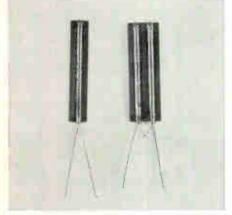
Weldable strain gages, one-piece, etched wire filaments in swaged stainless steel tubes, are suitable for use from cryogenic to elevated temperatures. Photo shows typical gages in actual size.
