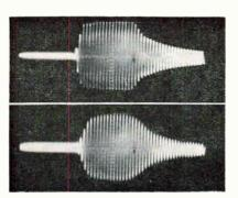
Upper oscillogram is the 10-Mc input to a shear-mode delay line, while the lower one shows the output delayed by 80 microseconds
