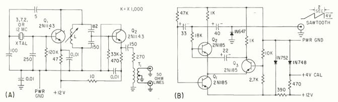
FIG. 2—Circuits used in standing-wave detector: oscillator (A) develops an r-f signal of one volt rms into two balanced transmission lines; generator (B) develops the linear sawtooth signal (shown) that is applied to antenna elements
