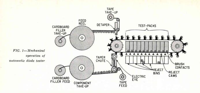
designed for in-line movement by a nylon conveyor belt. The conveyer is indexed in 3-in. increments by an 8-stop roller-gear indexing unit. The conveyer is driven by a 1-hp variable-speed drive coupled by a clutch and brake to the index unit.
