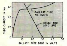
FIG. 2—Ballast tube has required characteristic for application
