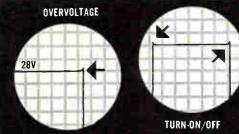
OVERVOLTAGE PROTECTION: Voltage excursion above operating voltage in case of internal fault condition is less than 5% or 1% volts for less than 5 milliseconds.
