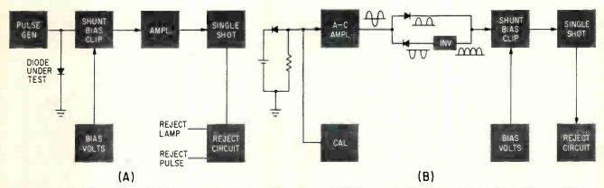
FIG. 4—Forward recovery circuit (A) compares pulse voltage drop across diode with preset reject voltage. Flutter tester (B) measures a-c component of fluctuating d-c produced by diode and battery in series
