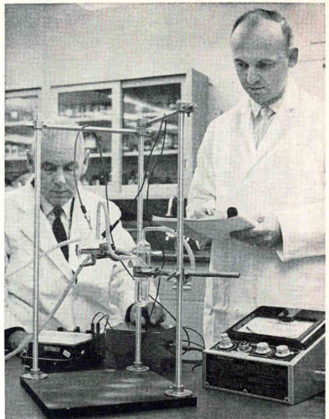
New ion-exchange cell, the size of a quarter, (left) produces slightly less than 1 volt and up to 100 amperes per sq ft. A number of these cells in series will power space equipment, telemetry devices, and portable ground communications, with efficiencies of 90 per cent. Inventors Dravnieks and Bregman (right) check voltages on experimental apparatus used during successful testing of the inorganic membrane
