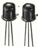
2N2187 Matched pair of Philco type 2N2185 SPAT Choppers, in TO-18 Packages.
