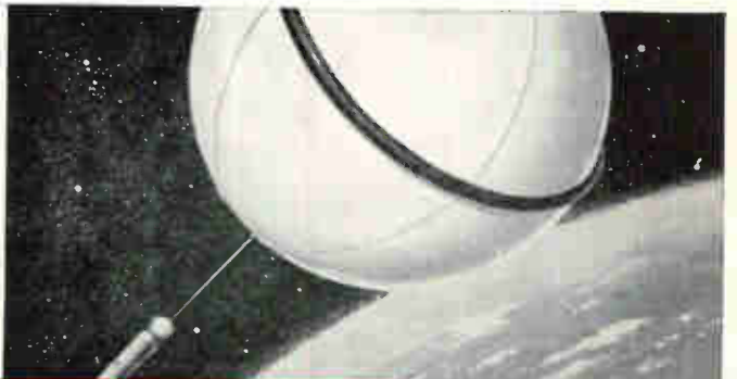
Ballute recovery system, tested and proven in flight test, provides variable controlled drag for re-entry vehicle.
