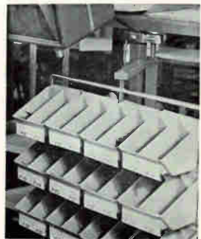
Swing-out bin frame allows each operator to adjust bins for easiest reaching
