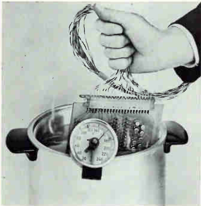
"NO POTS AT ALL" STABILITY of the NLS V44 digital voltmeter is checked by the "boil in oil" test at 158 F. This design feature eliminates all trimming of decade and amplifier circuits.
