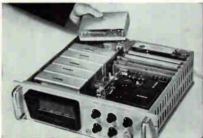
PLUG-IN OIL-BATH STEPPING SWITCHES in Series 30 instruments outlast dry switches by a factor of five... completely eliminate periodic disassembly for manual lubrication of switches... and permit replacing switches in several minutes for fast troubleshooting and repair.
