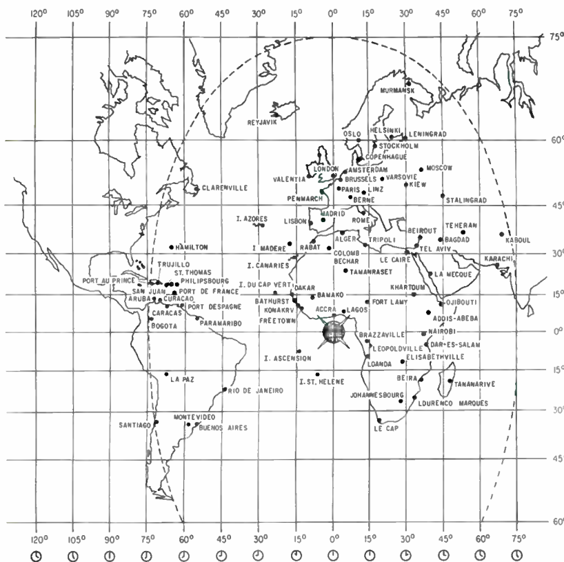
Satellite put into synchronized equatorial orbit would remain fixed with respect to earth, 22,400 miles above 0 deg latitude, 0 deg longitude. Dotted line shows where transmitting-receiving stations could be set up
