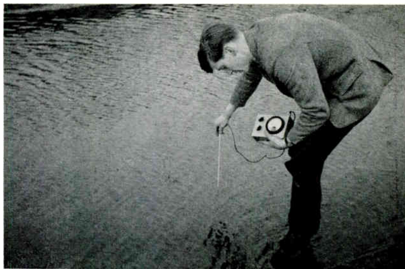
Measuring water velocity with portable propeller flowmeter
