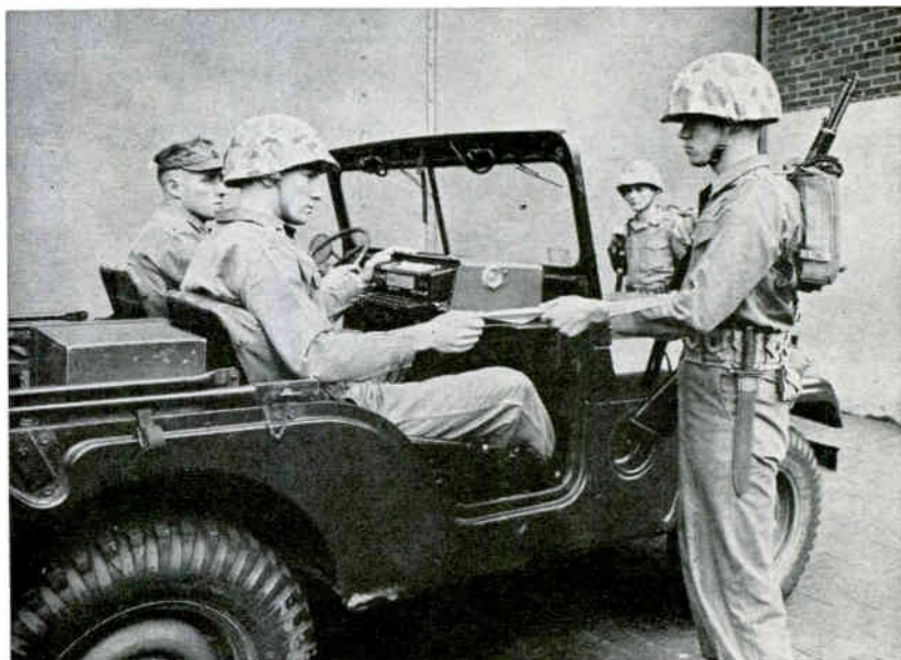
Designed for military service, teletypewriter by Mite Corp. uses solid state line sensing, operates to 100 words a minute
