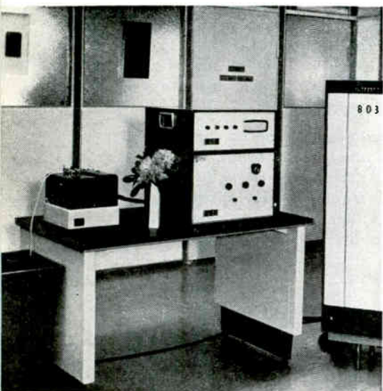
Neutron-time-of-flight analyzer and data processing setup
