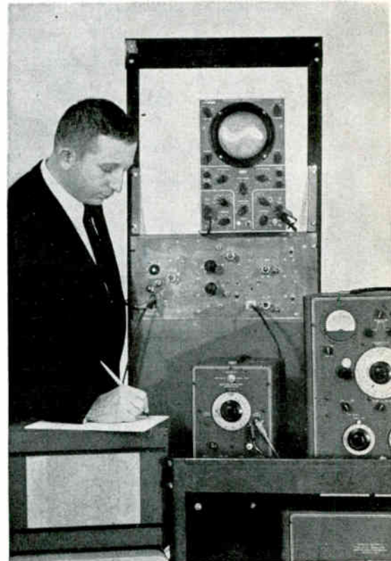
Staggered-tuned discriminator, shown with author, brings distortion below 0.25 percent for a frequency deviation of 40 Kc
