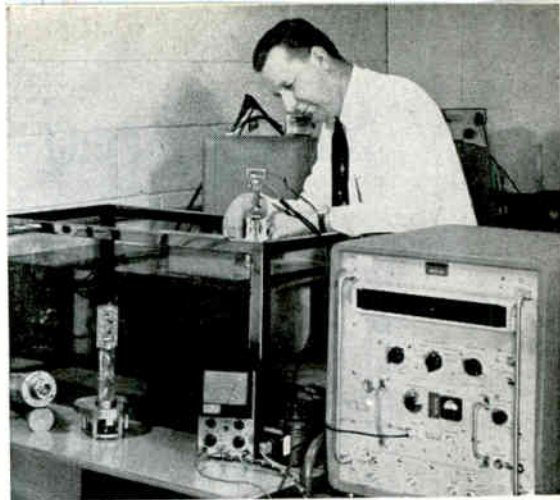
Watertight housing (left) shown removed from velocimeter built by ACF Electronics Div. Plate on spacers (bottom, same photo) protects transducers and reflectors from damage. Picture at right shows velocimeters undergoing tests at firm's laboratory. Readout is obtained on frequency counter
