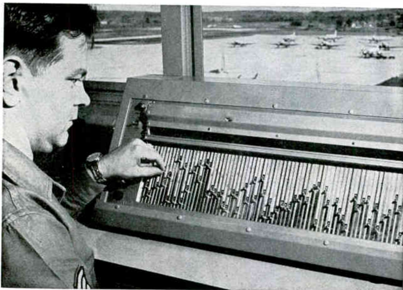
Air Force's new telecode weather transmitter under test. Temperature, wind direction, other variables are set on 72 metal slides. On pushbutton command, data is sent to remote weather stations
